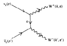
$$T\left(\nu\overline{\nu} \longrightarrow W^{+}W^{-}\right) = -i\overline{v}\left(p'\right)\left(-ig\varsigma'\right)\left(1-\gamma_{5}\right)\frac{i}{p'-k'-m_{e}}\left(-ig\varsigma'\right)\left(1-\gamma_{5}\right)u\left(p\right)$$
