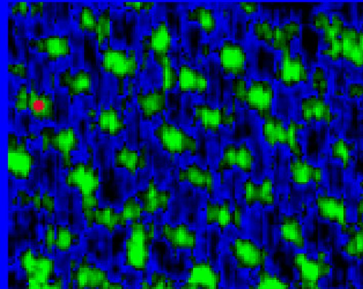
Field driven flux motion probed by STM on NbSe2
