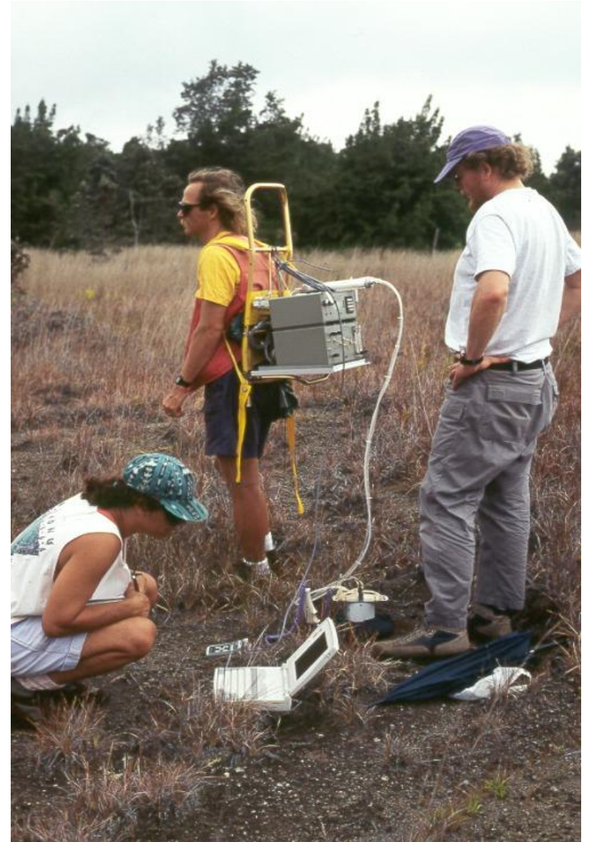
LI-COR analyzer on backpack, Kilauea Volcano
