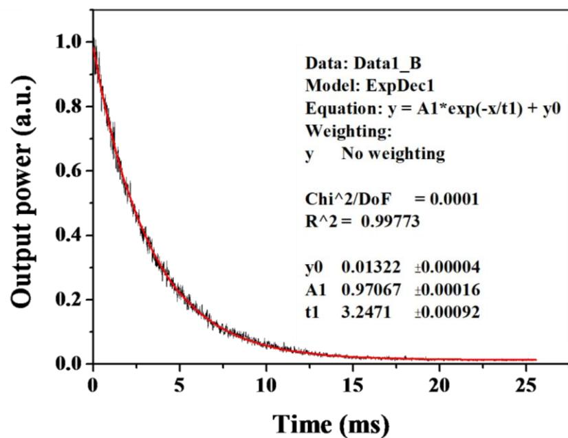
Exp. result: measured lifetime vs. pump
