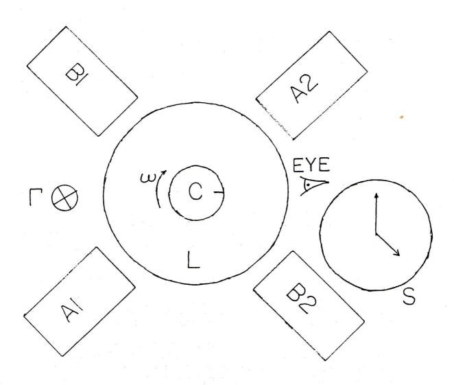
Figure 1 Open Loop System - A cylinder, C, is magnetically suspended in a liquid L. This shows a top view of the set up. Drive coil pairs Al-A2 and Bl-B2 create a rotating magnetic field which produces a torque,  $\Gamma$ , on the cylinder and causes it to rotate. The angular velocity of the cylinder,  $\omega$ , is recorded by eye and a stopwatch, S.  $\Gamma$  is into the page.
