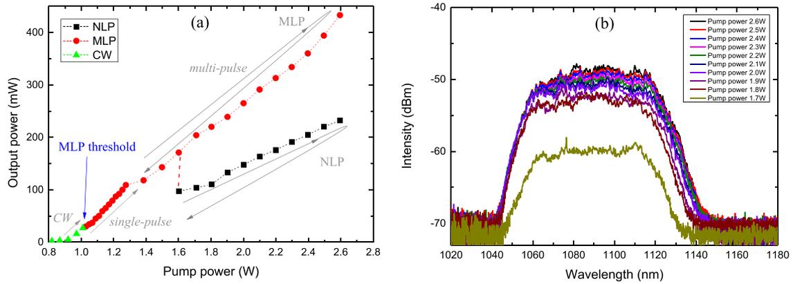
Fig. 2. (a) Operating regime of the laser as a function of pump power. CW, continuous wave; (b) Output spectra of the Laser operating in NLP mode. Traces of different color correspond to different pump power.
