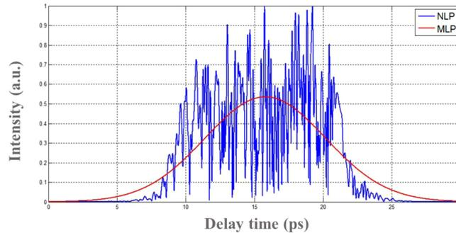
Fig. 5. Examples of simulated NLP and MLP waveforms of equal pulse energies and similar durations. NLP: noise-like pulses, MLP: mode-locked pulse.
