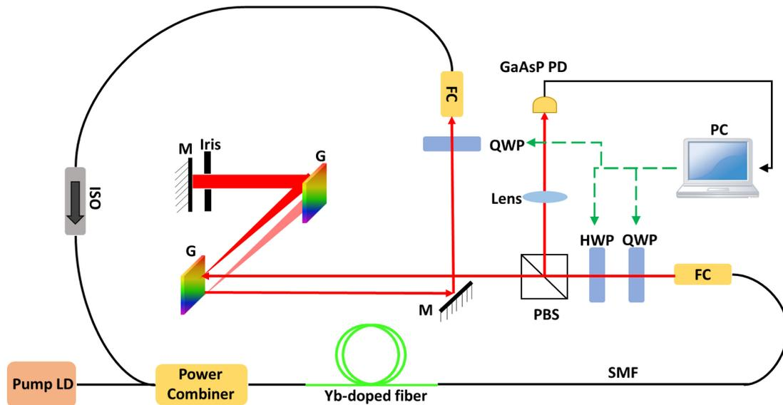
Fig. 1. Schematic setup of the fiber laser system. FC, fiber coupler; G, grating; HWP, half-wave plate; QWP, quarter-wave plate; PBS, polarization beam splitter; M, mirror; LD, laser diode; PC, personal computer.
