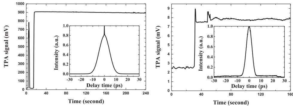
Fig. 6. TPA signals versus time for (a) the NLP and (b) the MLP. The insets are respectively their autocorrelation traces.
