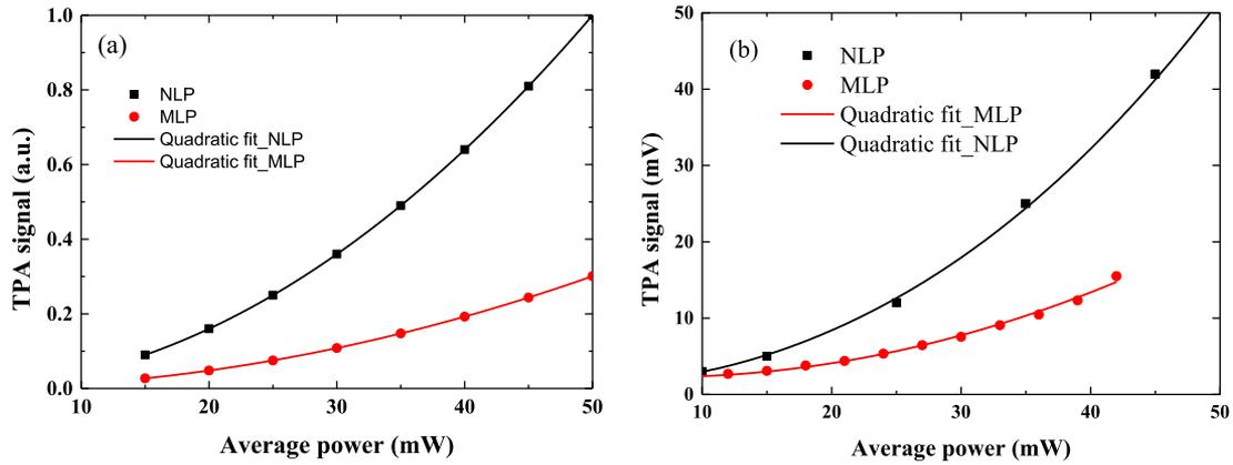
Fig. 4. The quadratic dependence of TPA signal as a function of the average power for the NLP and the MLP by (a) theoretical simulation and (b) experiment.
