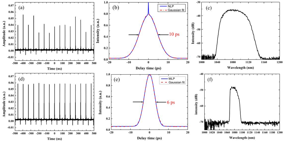
Fig. 3. Oscilloscope traces of the pulse trains, autocorrelation traces, and optical spectra of the laser operating in NLP (a, b, c) and (single-pulse) MLP (d, e, f) modes.
