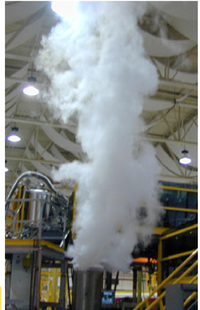
A magnet undergoing a controlled quench.
