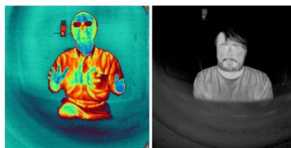
FIG. 4. (Color online) 80 K images taken with a 1024×1024 pixel SML QDIP FPA with f/2 optics.
