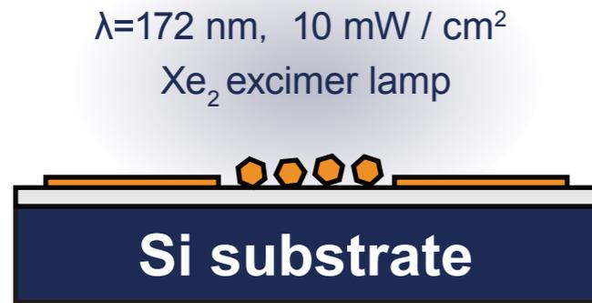
Prior to sonication, the sample was reduced by VUV irradiation.
