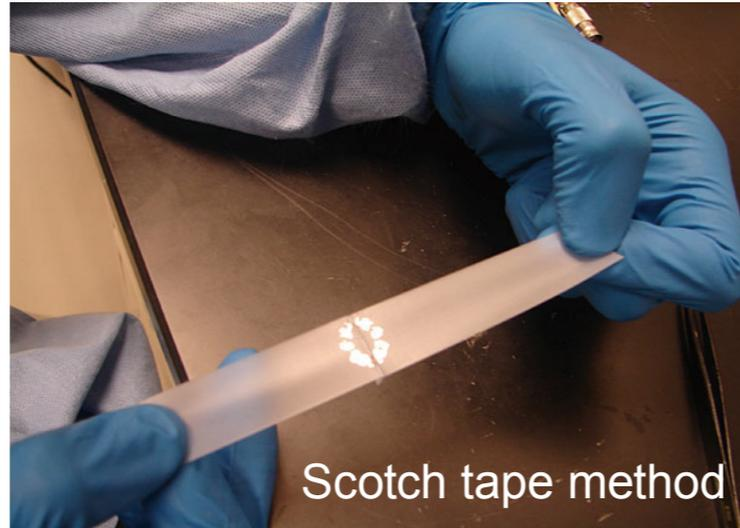
Mechanical cleavage: Scotch tape method
