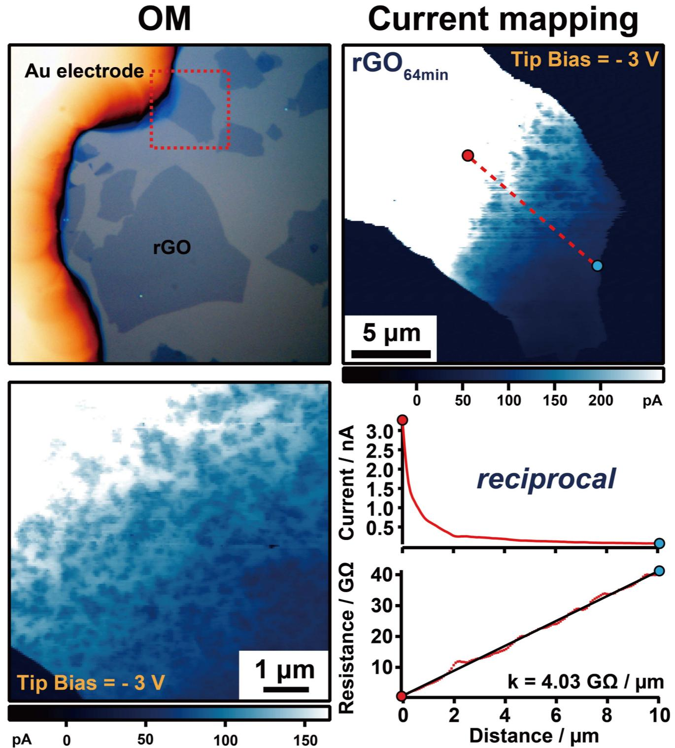
Sub- $\mu\text{m}$  conductive rGO lines were successfully fabricated in a sheet.
