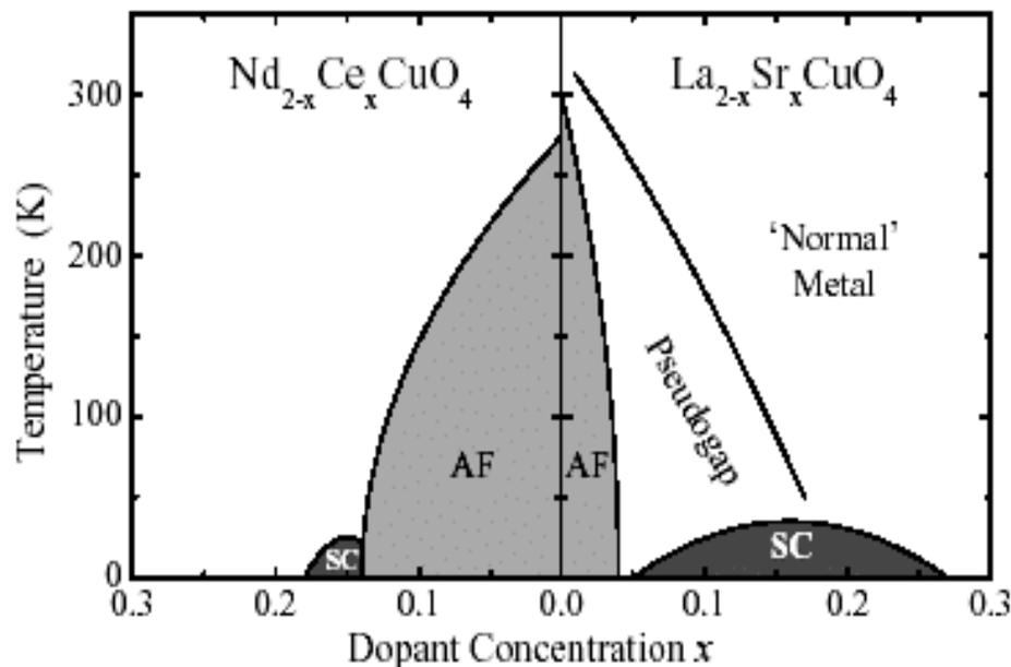
FIG. 1. Phase diagram of n and p-type superconductors.
