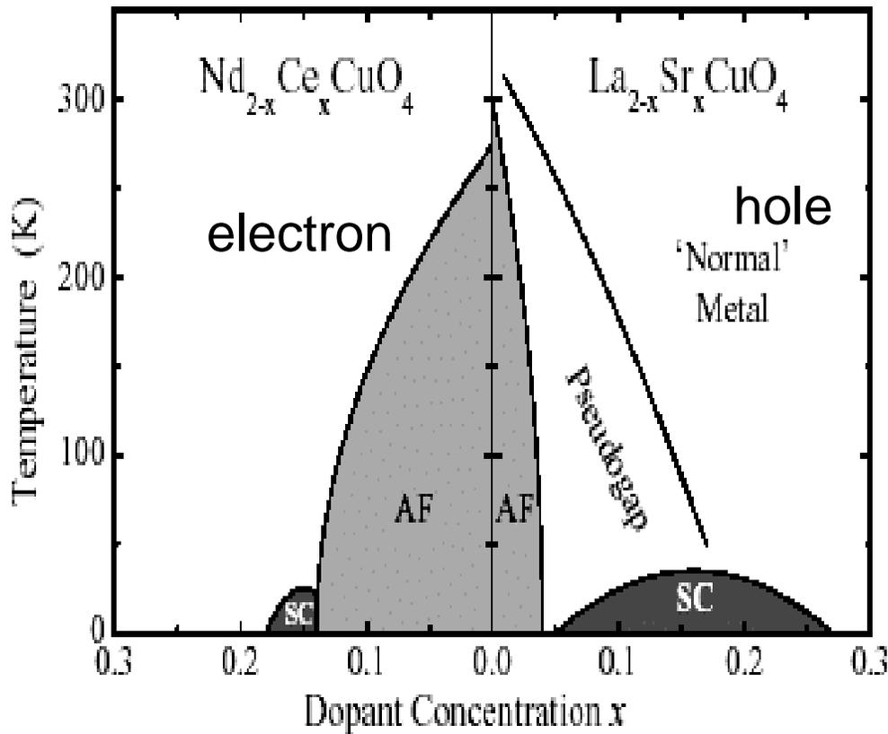
FIG. 1. Phase diagram of n and p-type superconductors.
