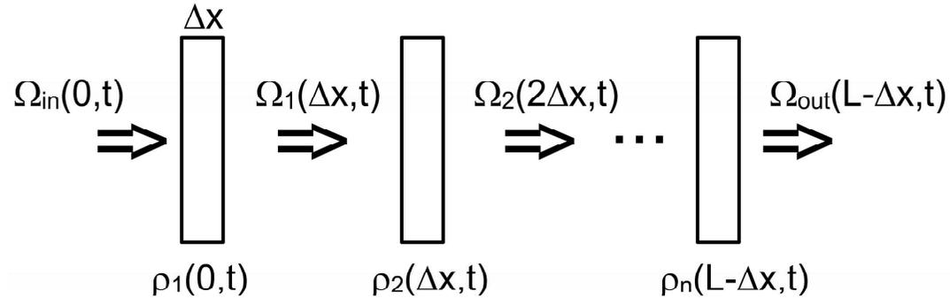
$$\Omega_{i+1}(x + \Delta x, t) = \Omega_i(x, t) \left\{ 1 - \frac{3\lambda^2 \Gamma N}{4\pi} \frac{Im[\rho_{31}(x, t)]}{\Omega_i(x, t)} \Delta x \right\}$$
