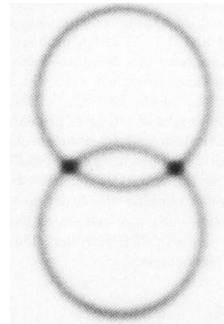
Down-conversion by a BBO crystal to generate two entangled photons along the intersecting directions of the cones.
