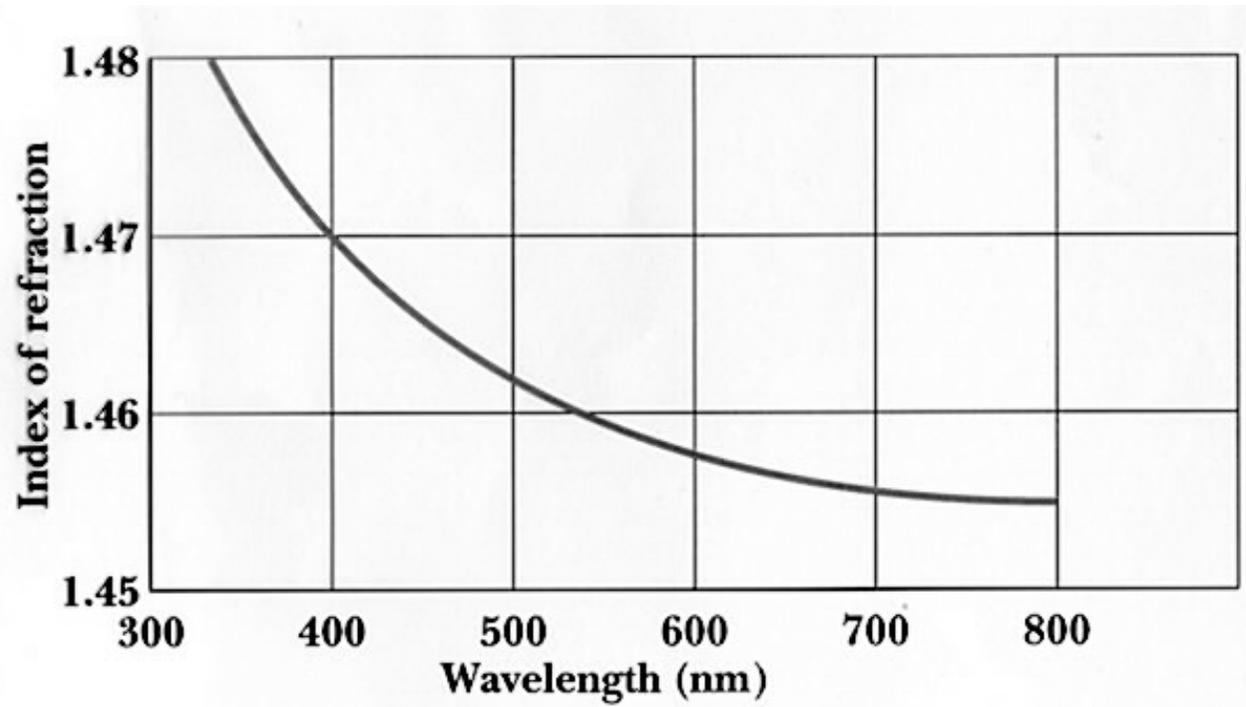
The index refraction of fused quartz.  $\omega \frac{dn}{d\omega} \approx 0.01$
