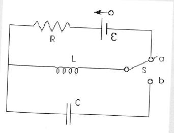
The switch has been in position *a* for a long time. The capacitor is uncharged.
