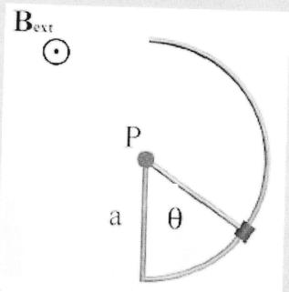
Consider the following pie shaped circuit. The arm is free to pivot about the center, P, and has mass *m* and resistance *R*.
