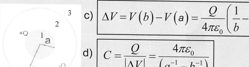
e) If you place an additional +2Q charge on the inner sphere then you will induce an additional -2Q on the inner surface of the outer shell, and hence a +2Q charge on the outer surface of that shell
