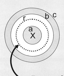
Everywhere the magnetic field is clockwise. To figure out the magnitude use Ampere's Law:
