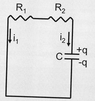
This is an easy circuit since it just looks like a resistor and capacitor in series, so:
