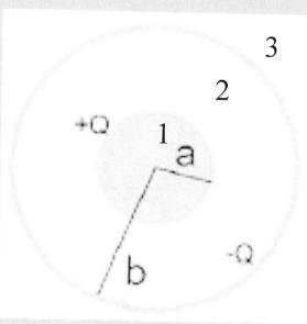
a) By symmetry **E** is purely radial. Choose spherical Gaussian surface
