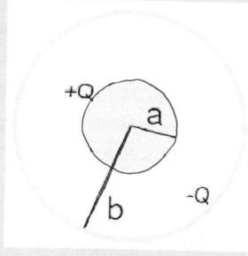
A conducting solid sphere of radius a, carrying a charge +Q is surrounded by a thin conducting spherical shell (inner radius b) with charge -Q.
