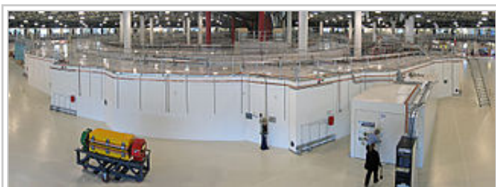
The interior of the Australian Synchrotron facility, a synchrotron light source. Dominating the image is the storage ring, showing a beamline at front right. The storage ring's interior includes a synchrotron and a linac.
