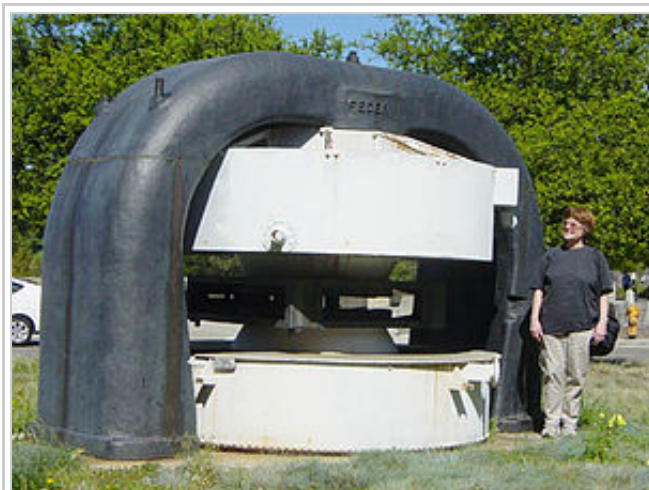
The magnet portion of a 27" cyclotron. The gray object is the upper pole piece, routing the magnetic field in two loops through a similar part below. The white canisters held conductive coils to generate the magnetic field. The D electrodes are contained in a vacuum chamber that was inserted in the central field gap.
