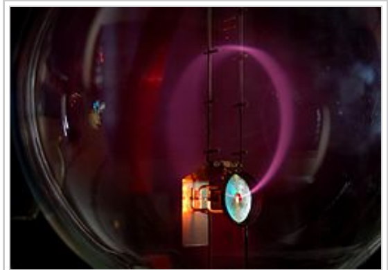
Beam of electrons moving in a circle. Lighting is caused by excitation of gas atoms in a bulb.
