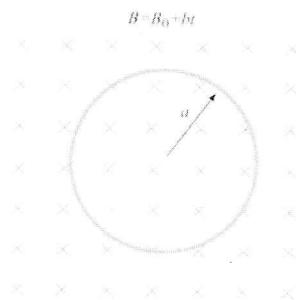
**Figure 10.9.5** Circular loop in a time-varying magnetic field
