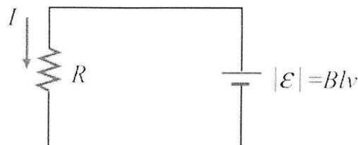
**Figure 10.2.3** Equivalent circuit diagram for the moving bar
