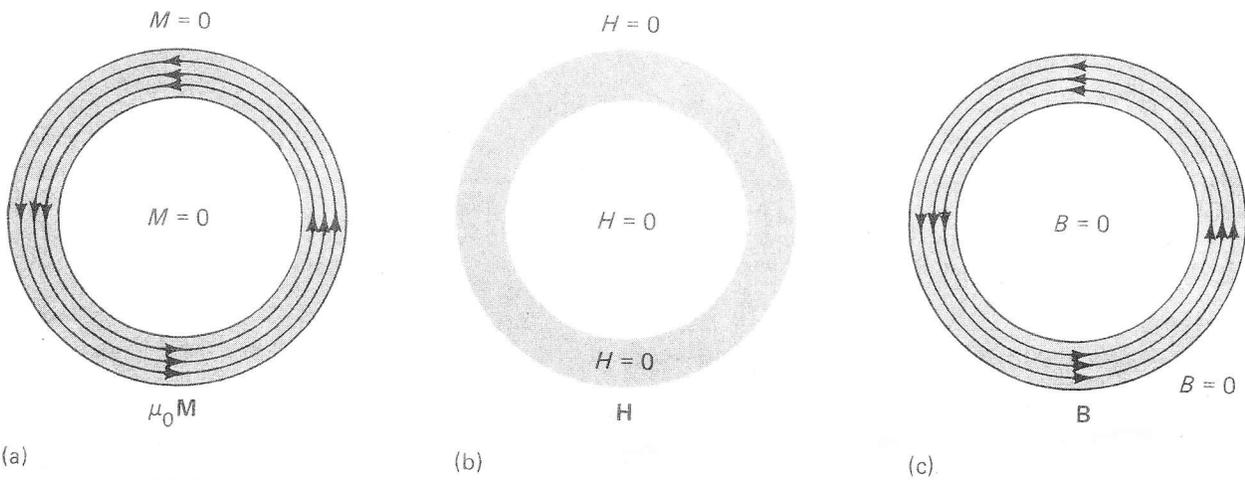
(a) Magnetization, (b) magnetic intensity, and (c) magnetic induction fields for a permanently magnetized toroidal sample.
