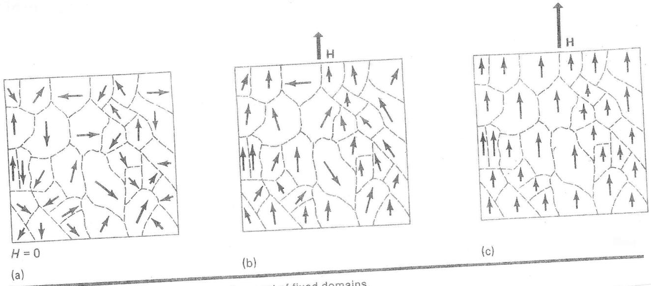
Magnetic alignment by alignment of fixed domains.
