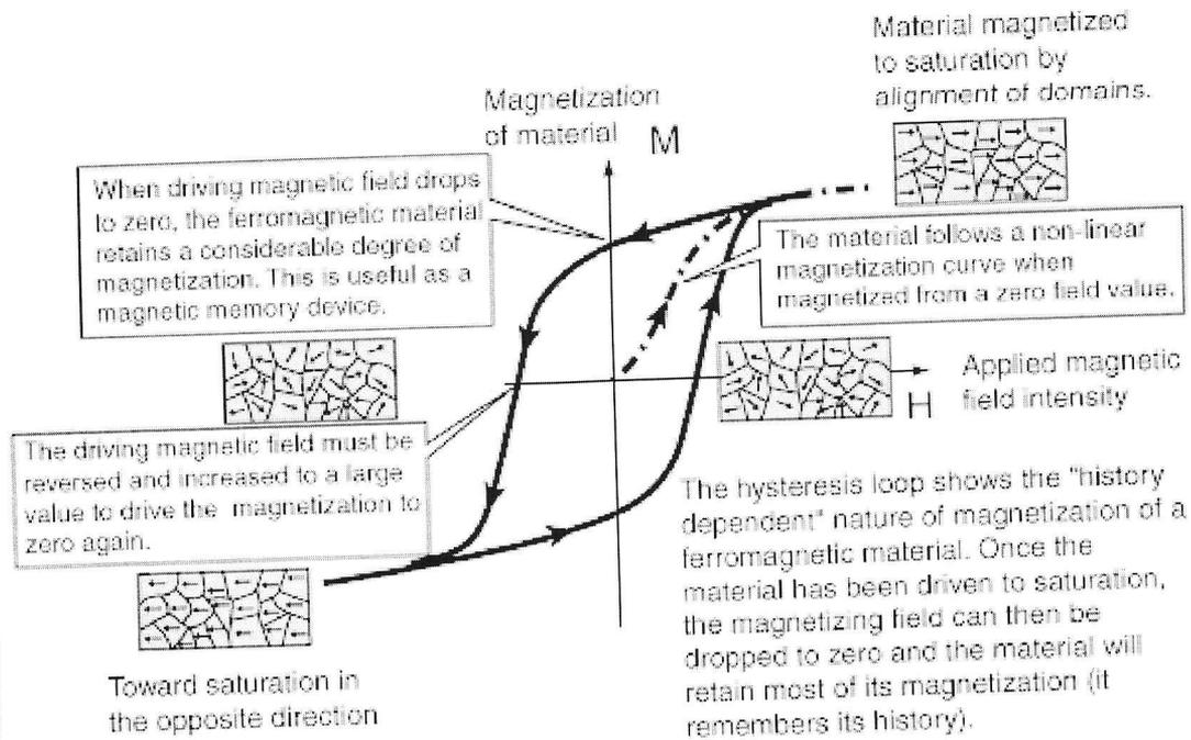
It is customary to plot the magnetization  $M$  of the sample as a function of the magnetic field strength  $H$ , since  $H$  is a measure of the externally applied field which drives the magnetization .
