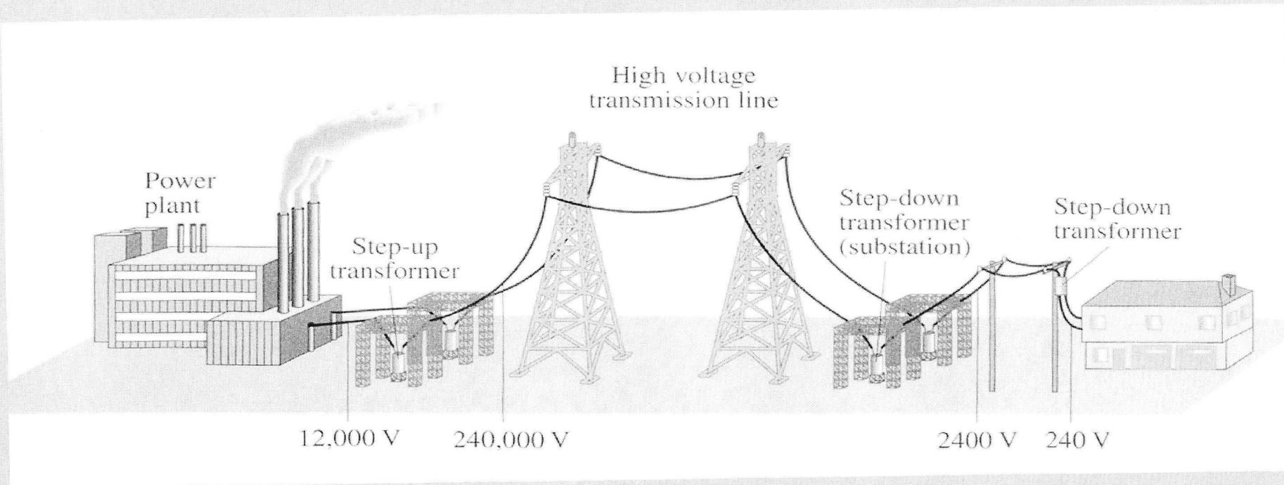
Power loss can be greatly reduced if transmitted at high voltage
