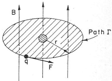
The induced electric forces on the electrons in an atom.
