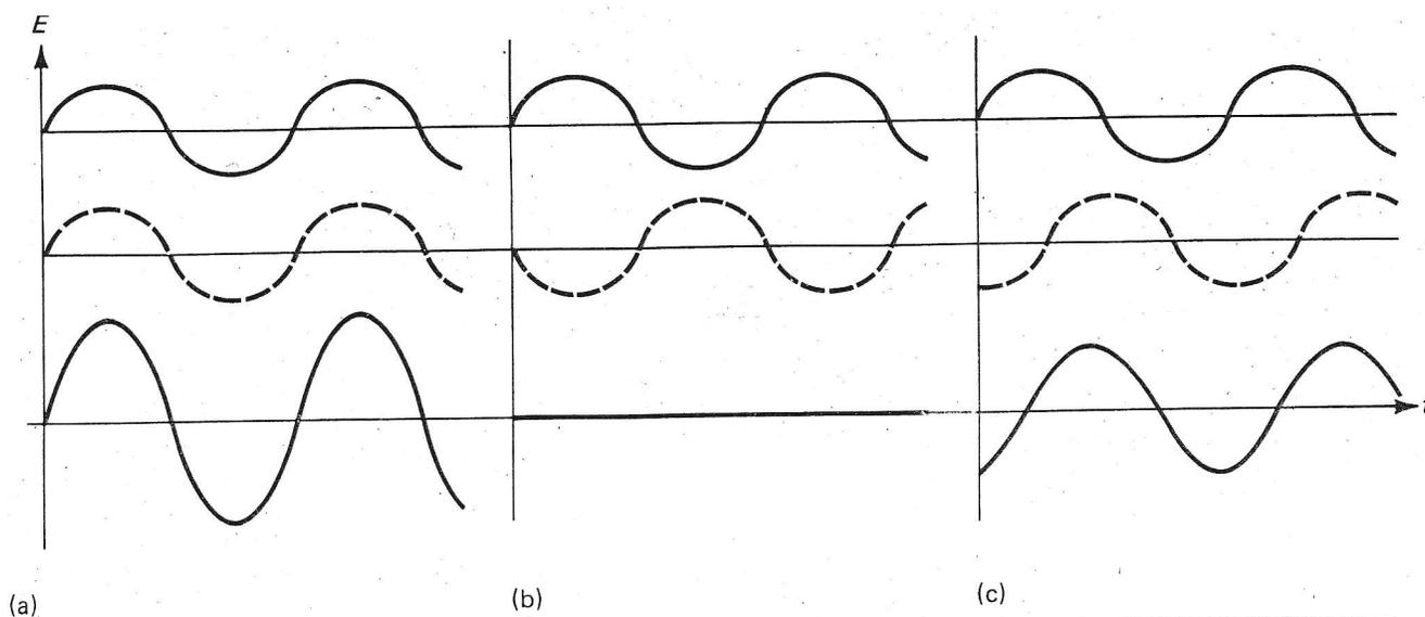
**FIGURE 26.8.** Superposition of plane waves (a) in phase, (b)  $180^\circ$  out of phase, and (c) with an intermediate phase difference.
