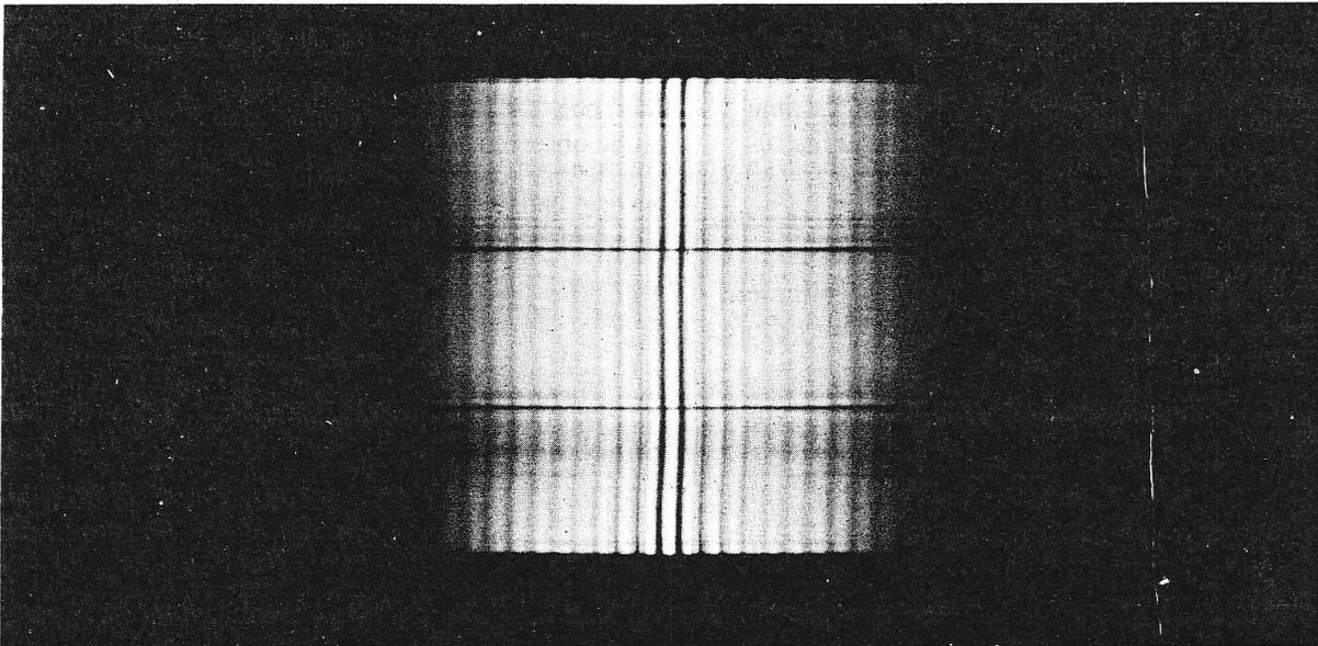
FIGURE 26.11. Photograph of double-slit interference fringes.
