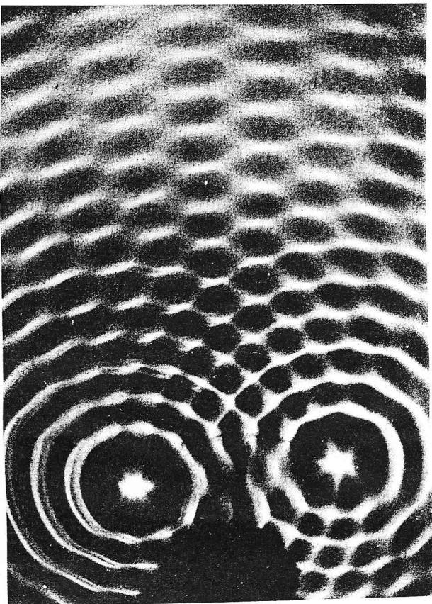
Interference of water waves from two coherent point sources. Photo courtesy of Professor T. A. Wiggins, Pennsylvania State University.
