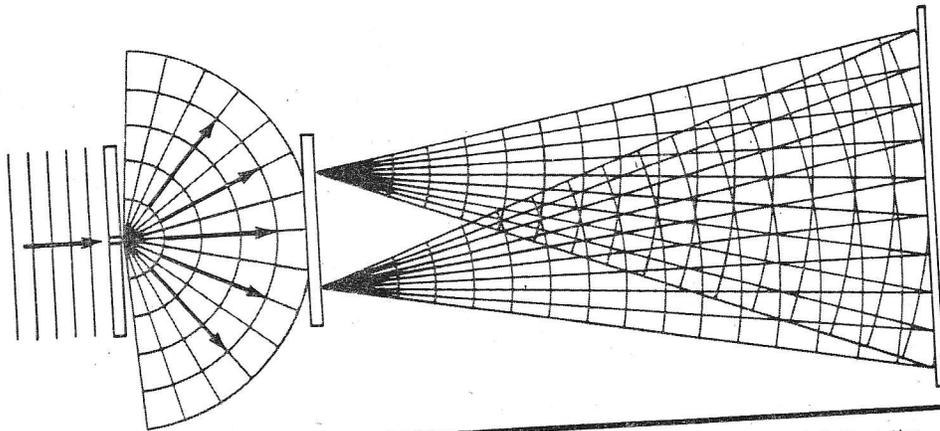
Diagram of rays and wavefronts in Young's experiment exhibiting the interference of light from two coherent point sources.
