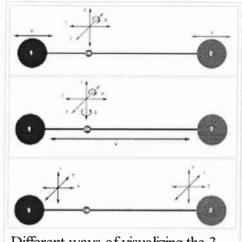
Different ways of visualizing the 3 degrees of freedom of a dumbbell-shaped diatomic molecule. (CM: center of mass of the system, T: translational motion, R: rotational motion, V: vibrational motion.)
