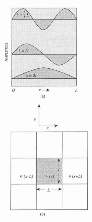
Figure 1.6: A schematic showing (a) the stationary boundary conditions applicable to a string clamped at x = 0 and x = L; and (b) periodic boundary conditions leading to plane wave solutions.
