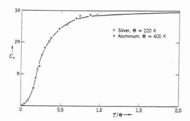
Heat capacity at constant volume as a function of temperature. The solid curve is the Debye function (eq. 8-17). The curve was fitted to the data points for each metal in order to determine the Debye temperature  $\Theta$  for the metal, and then the data were replotted as a function of  $T/\Theta$ . (From F. Seitz, Modern Theory of Solids, McGraw-Hill, New York, 1940.)
