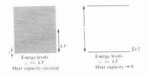
Fig. 6.1. Effect of energy-level spacing on heat capacities.
