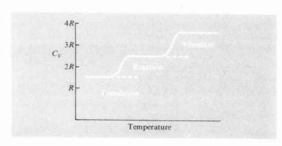
Fig. 6.2. Variation of heat capacity of a diatomic gas with temperature (only hydrogen isotopes give purely translation heat capacities).
