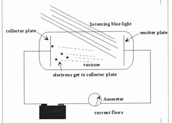
Question: In the above figure, the battery represents the potential Lenard used to charge the collector plate negatively, which would actually be a variable voltage source. Since the electrons ejected by the blue light are getting to the collector plate, evidently the potential supplied by the battery is less than  $V_{\rm stop}$  for blue light. Show with an arrow on the wire the direction of the electric current in the wire.
