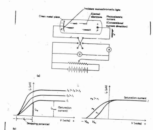
(a) Schematic for photoelectric experiment. (b) Photoelectric current versus the accelerating potential V for incident monochromatic light of wavelength  $\lambda$ . (c) Photoelectric current versus accelerating potential to show frequency dependence.
