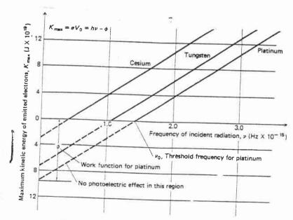
The maximum kinetic energy of photoelectrons  $K_{\max}$  (=  $eV_0$ ) versus the frequency of incident radiation.
