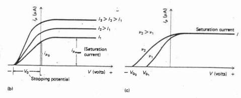
(a) Schematic for photoelectric experiment. (b) Photoelectric current versus the accelerating potential  $\mathcal V$  for incident monochromatic light of wavelength  $\lambda$ . (c) Photoelectric current versus accelerating potential to show frequency dependence.
