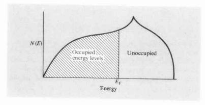
Fig. 6.6. A simple band diagram for a metal.
