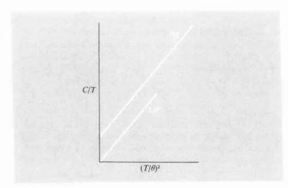
Fig. 6.5. Comparison of low-temperature heat capacities of a metal and an insulator.
