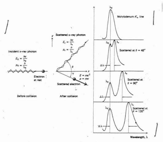
Compton scattering of a photon from an electron at rest. The graphs at the right show the shift in the  $K_{\bullet}$  radiation from molybdenum scattered from carbon.
