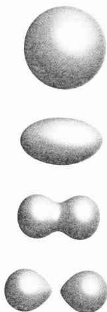
• Figure 15-7 The sequence of shapes assumed by a charged oscillating liquid drop. The last stage is at the point of fission into two smaller drops.
