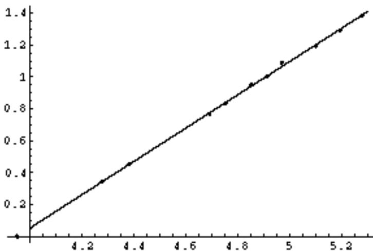
Comparing this with the thick plate, we see that the thick plate diverges from the ideal more than does the this plate. This data closely fits the straight line and shows that the frequency does vary as a function of  $(m^2 + n^2)^{\text{power}}$ . The slope of our line does not confirm that the power is  $1/2$ .
