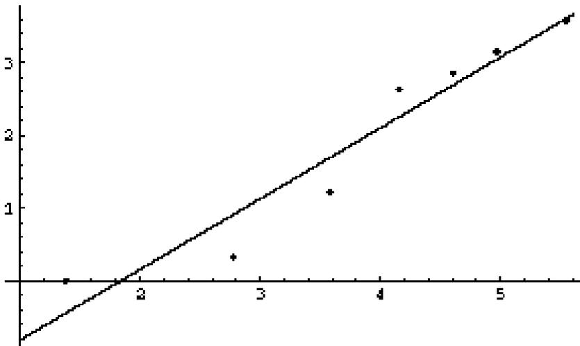
Note: Slope of this best fit line is about 1, which means data does not reflect Chladni's law. This data indicates that  $f/f_0 \sim (m+b*n)^k$  when  $k$  is around 1, not 2. This is not surprising, as Chladni's law applied to plates with fixed boundaries, unlike our experiment.
