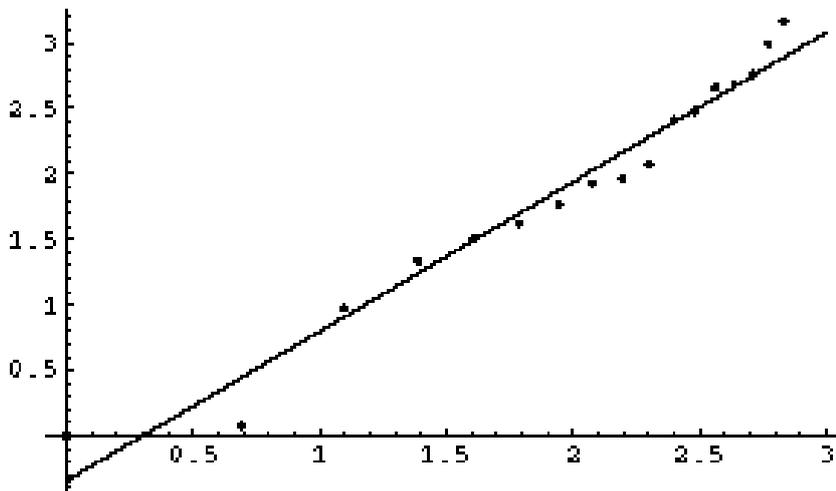
This matches theoretical prediction, but does not prove it. Since the plate is square, increasing  $m$  should have the same effect as increasing  $n$ . Thus, we can number the modes ordinally and still get a straight line. The graph shows that there is some power relation between the mode numbers and the frequency.
