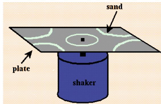
With this you can vibrate much larger plates to much higher and purer modes. The shape of the plate is important. The usual demonstrations are round and square plates. Here are some sample patterns: all the plates were 0.125 inch thick Aluminum, painted black.
