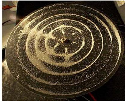
Notice the clear, distinct radial nodes while the diametric nodes are much more difficult to determine.
