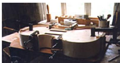
Before an instrument is glued together, the interior is sealed with a mineral paste comprising montmorillonite (bentonite) coloured light brown with walnut vegetable stain. Montmorillonite has very similar properties to the volcanic
