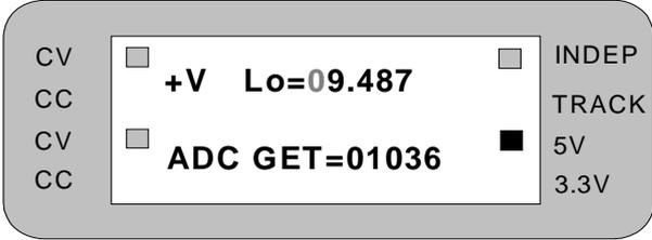
Step 2: Measure the DC voltage from the +output terminals (+ and COM1) with the DMM and key in the measured value (i.e. if the DMM shows 9.487V then key in 9.487) followed by the “ENTER” key. The following message will then appear on the LCD:
