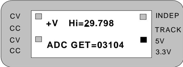
Step 3: Repeat step 2. Key in the measured value (i.e. if the DMM shows 29.798V then key in 29.798) followed by the “ENTER” key. The following message will then appear on the LCD.
