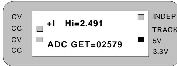
Step 5: Repeat step 4. Keyin the measured value (i.e. if the DMM shows 2.491A then keyin 2.491) followed by the “ENTER” key. The following message will then appear on the LCD:
