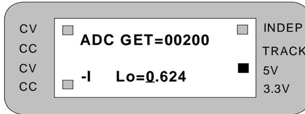
Step 8: Measure the DC current from –output terminals ( - and COM) with the DMM and keyin the measured value (i.e. if the DMM shows 0.642A then keyin 0.642) followed by the “ENTER” key.
