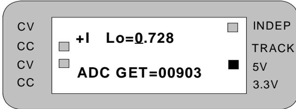
Step 4: Measure the DC current from +out terminals (+ and COM1) with the DMM and keyin the value (i.e. if the DMM shows 0.728A, then keyin 0.728 ) followed by the “ENTER” key. The following message will then appear on the LCD:
