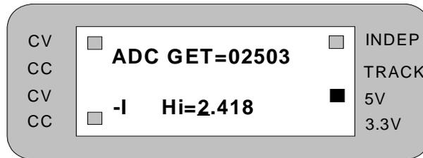
Step 9: Repeat step 8. Keyin the measured value (i.e. if the DMM shows 2.418A, then keyin 2.418) followed by the “ENTER” key. The following message will then appear on the LCD :
