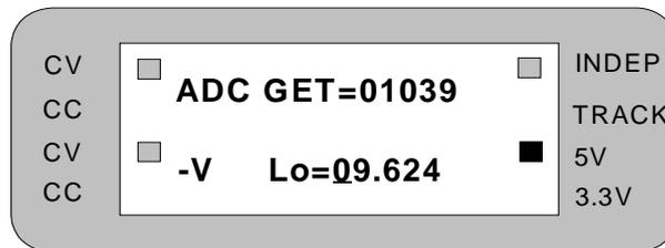
Step 6: Measure the DC voltage from –output terminals ( - and COM1) with the DMM and keyin the measured value (i.e. if the DMM shows 9.624V then keyin 9.624) followed by the “ENTER” key.
