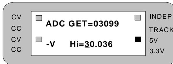
Step 7: Repeat step 6. Keyin the measured value (i.e. if the DMM shows 30.036V, then keyin 30.036) followed by the “ENTER” key. The following message will then appear on the LCD:
