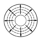
3. (20%) A coaxial cable usually works in the TEM mode with the fields
