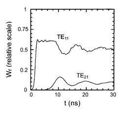
FIG. 37. Simulated evolution of the field energies of the  $TE_{21}$  and  $TE_{11}$  modes. The electron beam and a 450-W,  $TE_{11}$  drive wave are injected simultaneously at t=0. From Chu *et al.*, 1991.
