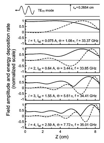
FIG. 28. Model and linear axial modes of a gyro-BWO. Top figure: the gyro-BWO interaction structure (a uniform wave-guide). Bottom figures: axial dependence of calculated field amplitude (solid curves) and beam energy deposition rate (dashed curves) of the first four axial modes at their respective  $I_{st}$ .  $V_b = 95 \, \mathrm{kV}$ ,  $\alpha = 1.1$ ,  $r_c = 0.35 \, r_w$ , and  $B_0 = 14.5 \, \mathrm{kG}$ . From Chen *et al.*, 2002.
