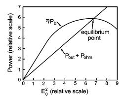
FIG. 26. Schematic illustration of the beam-generated power  $(\eta P_b)$  and the sum of output and Ohmic powers  $(P_{out} + P_{ohm})$  as functions of the square of the field amplitude  $(E_0^2)$ .  $E_0$  increases when  $\eta P_b > P_{out} + P_{ohm}$  and decreases when  $\eta P_b < P_{out} + P_{ohm}$ . Hence a stable equilibrium is maintained at the intersection of the two curves, which is usually designed to occur at or near the maximum efficiency point.
