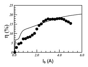
FIG. 49. Output power (normalized to the beam power) of gyro-BWO at the upstream port as a function of the beam current: ●, measured power; solid curve, calculated power. Measured and calculated powers at the downstream port (not shown) are negligible by comparison. Stationary oscillations have been observed at all operating currents. Parameters are the same as in Fig. 47. From Chang *et al.*, 2001.
