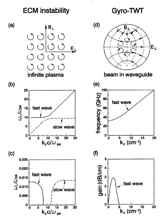
FIG. 20. Comparison of the ECM as a plasma instability [(a)-(c)] and as a radiation source [the gyro-TWT, (d)-(f)] in terms of the dispersive media [(a) and (d)], dispersive properties [(b) and (e)], and growth spectra [(c) and (f)]. The TE<sub>11</sub>-mode dispersion curve shown in (e) is for a waveguide radius of 0.266 cm.
