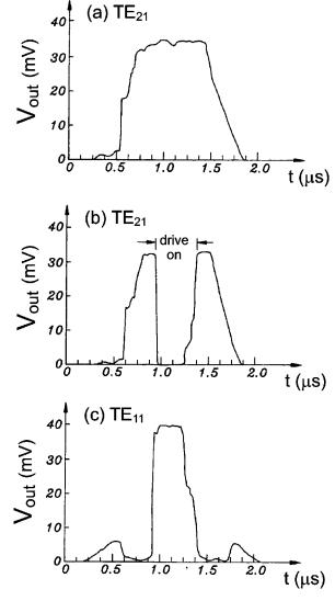
FIG. 34. Oscilloscope traces showing oscillation suppression by a large-amplitude drive wave: (a)  $TE_{21}$  oscillation signal at zero drive over the duration of the beam pulse; (b)  $TE_{21}$  oscillation signal with a 1-kW,  $TE_{11}$  drive pulse applied in the middle of the beam pulse; (c)  $TE_{11}$  output signal during application of the 1-kW drive wave. Other experimental parameters are given in Fig. 33. From Chu *et al.*, 1991.
