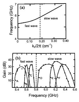
FIG. 16. Electron cyclotron maser instability in a dielectric loaded waveguide at  $I_b = 5$  A under different combinations of cathode voltage and magnetic field: (a) measured TE<sub>01</sub> dispersion curve; (b) small-signal gain. Curve A, 34 kV, 1.90 kG; curve B, 39.7 kV, 1.95 kG; curve C, 39.7 kV, 2.0 kG; curve D, 42 kV, 2.06 kG; curve E, 42 kV, 2.12 kG; curve F, 45.4 kV, 2.17 kG. Adapted from Guo *et al.*, 1982.
