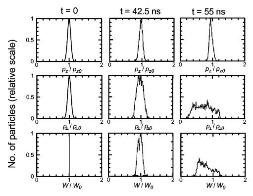
FIG. 36. Diagnostics of the electron distribution for the simulation in Fig. 35. The electron distribution at the end of the interaction section is diagnosed as a function of  $p_z/p_{z0}$ ,  $p_\perp/p_{\perp0}$ , and  $W/W_0$ , at times t=0, 42.5 ns, and 55 ns. From Chu *et al.*, 1991.
