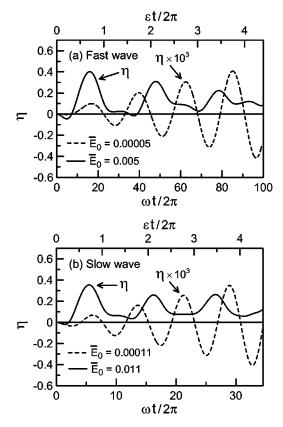
FIG. 8. Numerically evaluated interaction efficiency as a function of time in small-signal (dashed curve) and large-signal (solid curve) rf fields.  $V_b = 50 \, \mathrm{kV}$  for all runs: (a) fast-wave interaction,  $\omega/k_z = 2 \, c$  and  $\varepsilon/\omega = 0.044$ ; (b) slow-wave interaction,  $\omega/k_z = 0.5 \, c$  and  $\varepsilon/\omega = -0.12$ .
