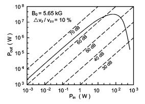
FIG. 23. Calculated gyroklystron output power vs input power for the parameters shown in Tables IV and V. From Chu *et al.*, 1985.
