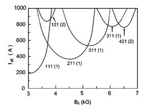
FIG. 24. Calculated start-oscillation current ( $I_{st}$ ) vs the magnetic field ( $B_0$ ) for modes with low  $I_{st}$  in the output cavity of Fig. 21. Mode indexes are labeled for each curve and the cyclotron harmonic number is indicated in parentheses. Dimensions of the cavity are given in Table III (cavity 4). Electronbeam parameters are given in Table IV. All modes have the same axial index of 1 and are assumed to have the same loaded O value of 100. From Chu *et al.*, 1985.
