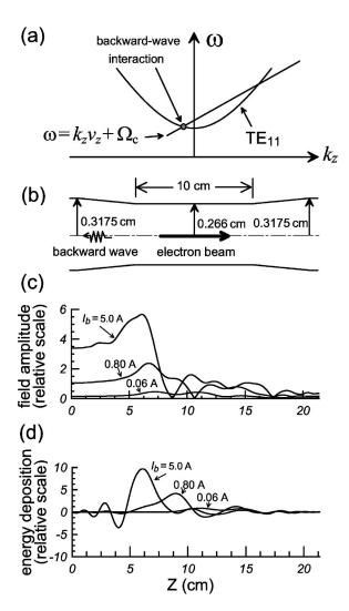
FIG. 47. Model and calculated behavior of a gyro-BWO: (a) operating point of the gyro-BWO in the  $\omega$ - $k_z$  diagram; (b) same interaction structure as in Fig. 46(b); (c) calculated linear and nonlinear field profiles at different  $I_b$ . (d) Calculated beam energy deposition profiles for the corresponding fields shown in (c). A cold electron beam is assumed.  $V_b$ =100 kV,  $\alpha$ =1,  $r_c/r_w$ =0.35, and  $B_0$ =14.59 kG. From Chang *et al.*, 2001.
