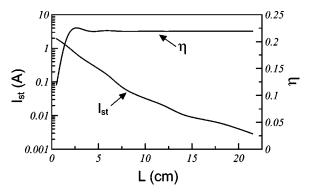
FIG. 43. Calculated start-oscillation current  $(I_{st})$  and nonlinear interaction efficiency  $(\eta)$  vs the uniform section length (L). The start-oscillation current depends sensitively upon L, whereas the nonlinear interaction efficiency (all evaluated at the beam current of 5 A) is almost independent of L as long as L exceeds a relaxation value of  $\sim$ 3 cm (cf. Fig. 45). Other parameters are the same as in Fig. 42. From Chen, Chu, and Chang, 2000.
