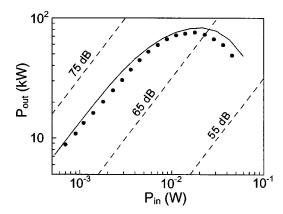
FIG. 41. Output power vs drive power at 34.2 GHz: dots, measured; solid curve, calculated. Other parameters are the same as in Fig. 40. From Chu *et al.*, 1998, 1999.
