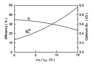
FIG. 22. Calculated gyroklystron efficiency as a function of the electron velocity spread. The optimum magnetic field varies with the velocity spread. From Chu *et al.*, 1985.
