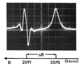
FIG. 14. Measured absorption coefficient vs magnetic field. Resonant magnetic fields for the fast ( $\gamma$ =1.01) and slow ( $\gamma$ ≈1) electrons differ by  $\Delta B/B_0$ ≈1%, consistent with the 1% difference in electron relativistic masses. From Hirshfield and Wachtel, 1964.
