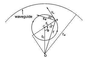
FIG. 12. Model of harmonic cyclotron interactions:  $E_{\theta}$ , electric field of the  $\text{TE}_{on}$  mode of a circular waveguide; O, center of the waveguide; C, center of electron gyration (guiding center).
