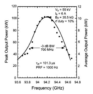
FIG. 25. Measured peak and average output powers (dots) of a five-cavity gyroklystron amplifier. The theoretical prediction (solid curve) assumes an  $\alpha (=v_{\perp 0}/v_{z0})$  value of 1.2 and an rms velocity spread of 3%. From Blank, Felch, *et al.*, 2002.
