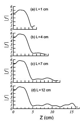
FIG. 44. Calculated nonlinear field profiles (relative scale, plotted from  $z_1$  to  $z_2$  of Fig. 42) for  $I_b$ =5 A and (a) L=1 cm; (b) L=4 cm; (c) L=7 cm; and (d) L=12 cm. Other parameters are the same as in Fig. 42. From Chen, Chu, and Chang, 2000.
