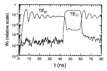
FIG. 35. Simulated evolution of the total field energy of  $TE_{21}$  and  $TE_{11}$  modes. The electron beam is injected at t=0. A 900-W,  $TE_{11}$  drive wave is injected at t=42.5 ns and turned off at t=58 ns. Other parameters are the same as in Fig. 33. From Chu *et al.*, 1991.
