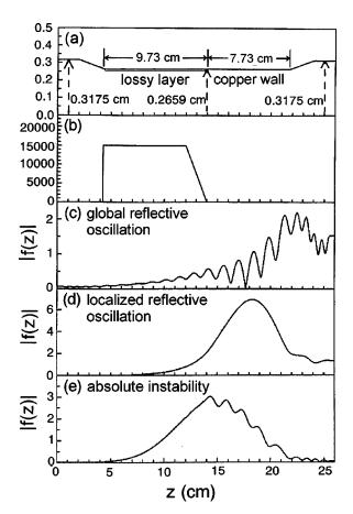
FIG. 39. Calculated rf field profiles, |f(z)|, of three types of oscillations in a distributed-loss structure: (a) and (b), the structure; (c) global reflective oscillation of the  $TE_{11}$  mode; (d) localized reflective oscillation of the  $TE_{11}$  mode; (e) the  $TE_{21}$  absolute instability. Operating parameters in (c)–(e) were chosen to accentuate the respective types of oscillations. From Chu *et al.*, 1998, 1999.
