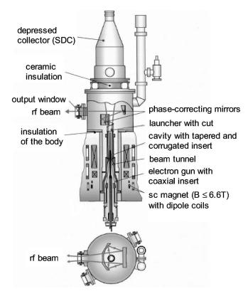
FIG. 27. Schematic layout of an 165-GHz,  $TE_{31,17}$ -mode, 2.2-MW coaxial gyromonotron. The insert at the bottom shows the quasioptical output coupling structure. From Piosczyk *et al.*, 2002.
