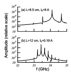
FIG. 53. Calculated output spectrum of a gyro-BWO at a beam current slightly above the onset current of the nonstationary state shown in Fig. 52: (a)  $L=8.5 \,\mathrm{cm}$ , (b)  $L=12 \,\mathrm{cm}$ . Other parameters are the same as in Fig. 28. From Chen *et al.*, 2002.
