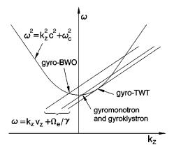
FIG. 19.  $\omega$  vs  $k_z$  diagram showing the intersection point between the mode line and the beam-wave synchronism lines for different types of gyrotrons.  $\omega_c$  denotes the cutoff frequency of the waveguide. For the resonant rf structures employed in the gyromonotron and gyroklystron,  $k_z$  assumes discrete values.
