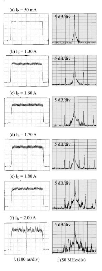
FIG. 50. Signal traces and corresponding spectrograms of gated gyromonotron output at different beam currents. Adapted from Chang *et al.*, 2001.
