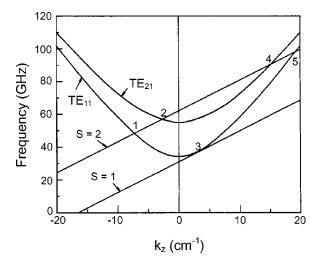
FIG. 30. Frequency vs  $k_z$  diagram of a fundamental cyclotron harmonic, Ka-band gyro-TWT based on the  $TE_{11}$ -mode convective instability (point 3). Other convective instabilities (points 4 and 5) and possible absolute instabilities (points 1 and 2) due to second cyclotron harmonic interactions are also indicated. This illustration assumes  $r_w$ =0.2654 cm,  $V_b$ =87.75 kV,  $\alpha$ =1, and  $B_0$ =12.38 kG.
