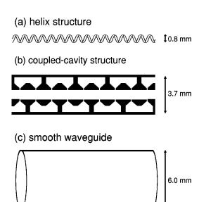
FIG. 1. Comparison of the shapes and transverse dimensions of three types of interaction structures: (a) a helix traveling-wave tube (TWT) structure; (b) a coupled-cavity TWT structure; and (c) a smooth waveguide, all at the operating frequency of 30 GHz in the lowest-order mode. From Chu, 2002.
