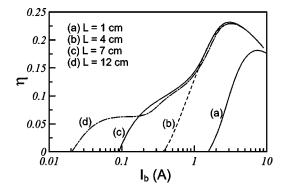
FIG. 45. Calculated efficiency vs beam current for different values of L. Oscillations start at widely different currents, but exhibit almost the same nonlinear behavior as long as L exceeds the relaxation length of  $\sim$ 3 cm. Other parameters are the same as in Fig. 42. From Chen, Chu, and Chang, 2000.
