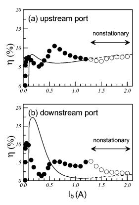
FIG. 48. Output power (normalized to the beam power) of a gyromonotron at (a) the upstream port and (b) the downstream port as functions of the beam current: ●, measured power in the stationary state; ○, measured power in the non-stationary state; solid curve, calculated power for the stationary state; dashed curve, calculated power for the nonstationary state. Parameters are the same as in Fig. 46. From Chang *et al.*, 2001
