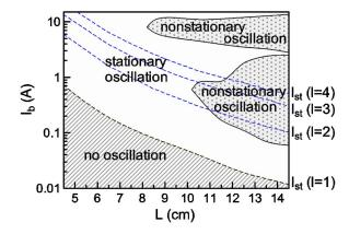
FIG. 52. Simulated stability map of a gyro-BWO with a uniform interaction structure of length L. Multiple nonstationary zones appear in the  $I_b$ -L space. No correlation is seen between the onset current of the nonstationary state and that of any higher-order axial mode (dashed curve). Other parameters are the same as in Fig. 28. From Chen *et al.*, 2002.
