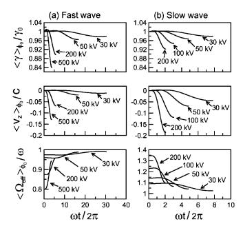
FIG. 11. Time dependence of the ensemble average of  $\gamma$ ,  $v_z$ , and  $\Omega_{\rm eff}$  for different electron energies at their respective optimum  $\varepsilon/\omega$  shown in Fig. 10. (a)  $\omega/k_z=2~c$ . (b)  $\omega/k_z=0.5~c$ . Each curve is terminated at the saturation time.
