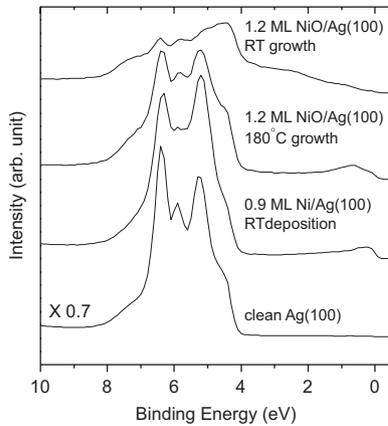
Fig. 1. AIPES of clean Ag(100), 0.9 ML NiO/Ag(100) as well as 1.2 ML NiO/Ag(100) grown at 180 °C and at RT with post annealing, all taken spectra at normal emission using HeII<sub>2</sub> at RT.
