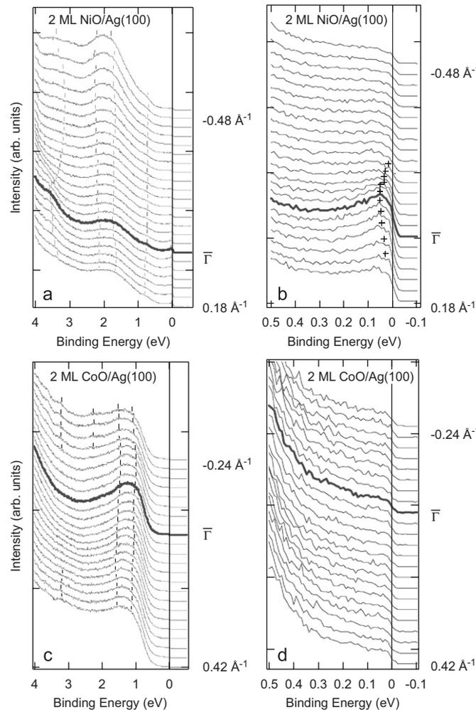
Fig. 2. ARPES spectra of (a) the valence band of 2 ML NiO/Ag(100) grown at RT also (b) the enlarged region near the Fermi level for (a), (c) valence band of 2 ML CoO/Ag(100) grown at 180 °C and (d) the enlarged region near the Fermi level for (c). The measurement is along  $\bar{\Gamma}-\bar{M}$  direction, where  $\bar{M}$  is referred to the  $(1 \times 1)$  Ag surface Brillouin zone. All spectra were taken at 51 eV photo energy.
