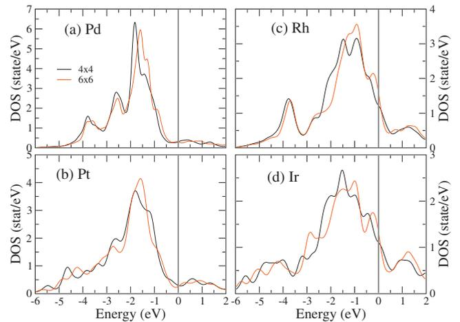
FIG. 4. (Color) Projected density of states of the topmost atom on  $4 \times 4$  (black lines) and  $6 \times 6$  (red lines) pyramids covered with one monolayer (a) Pd, (b) Pt, (c) Rh, and (d) Ir.
