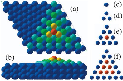
FIG. 1. (Color) Lattice structure of noble-metal covered W(111) single-atom tip. (a) Top and (b) side views of the  $6 \times 6$  three-sided pyramid structure. Red, yellow, green, and light blue spheres denote the first, second, third, and fourth layer atoms of the pyramid. Blue spheres are the tungsten atoms. [(c)–(f)] Atomic model of the topmost four layers of the pyramid. Blue and red balls denote the noble metal and tungsten atoms, respectively.
