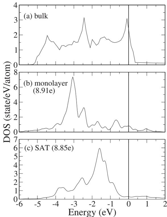
FIG. 2. The origin of the tip states in the Pd-covered single-atom tip. (a) DOS of bulk Pd. (b) DOS of monolayer Pd/W(111). (c) DOS of the tip Pd atom of SAT. The integrated valence charge of monolayer and SAT systems are also indicated in the brackets.
