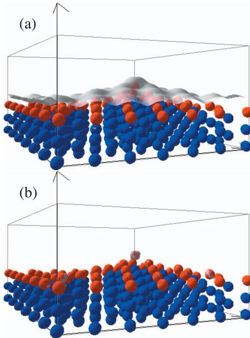
FIG. 3. (Color) (a) Charge contour (gray) of the itinerant states at Fermi level ( $0 \sim -0.4$  eV). (b) Charge contour (gray) of the localized tip states within ( $-1.4 \sim -1.8$  eV). Red and blue spheres denote the Pd cover layer and the W atoms, respectively.
