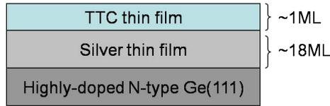
Figure 3.5: The growth model in this experiment, and the target thickness is shown on the scheme.
