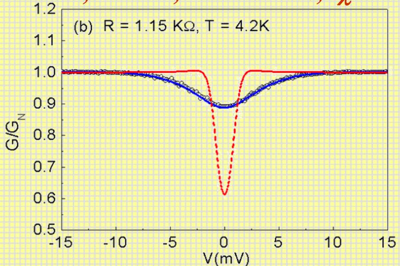
**Black open circles with spreading resistance fits (blue solid lines) and the extracted PCAR spectra (red dashed line) after removing the contribution of spreading resistances in**
