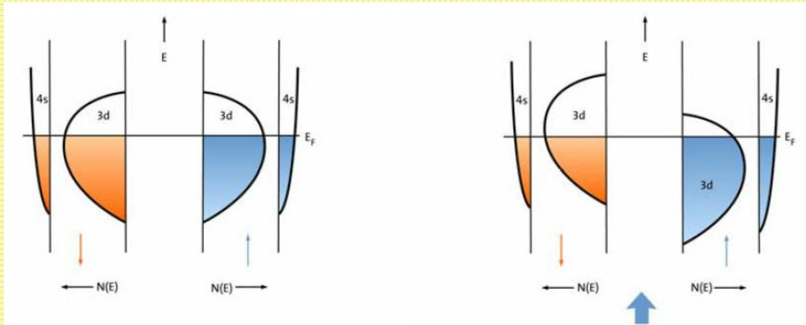
For the non-magnetic state there are identical density of states for the two spins.
