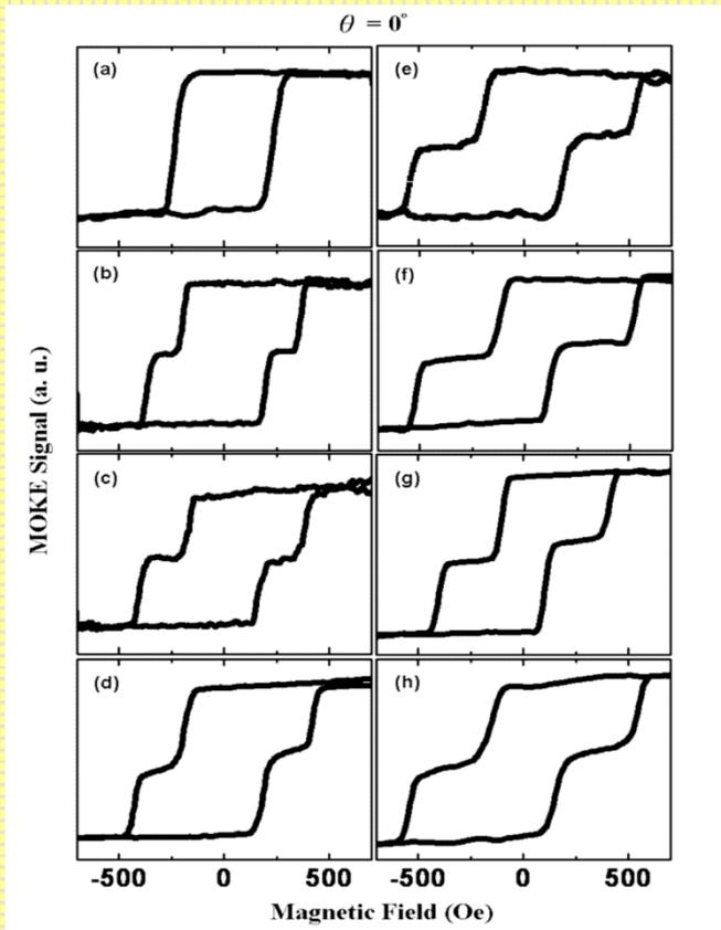
**Figure 2. [(a)-(h)] The MOKE signals for 20 nm NiFe elliptical rings arrays of fixed width 100 nm and circumference  $6.3\mu\text{m}$  for applied field parallel to the long axis of varied aspect ratios.**
