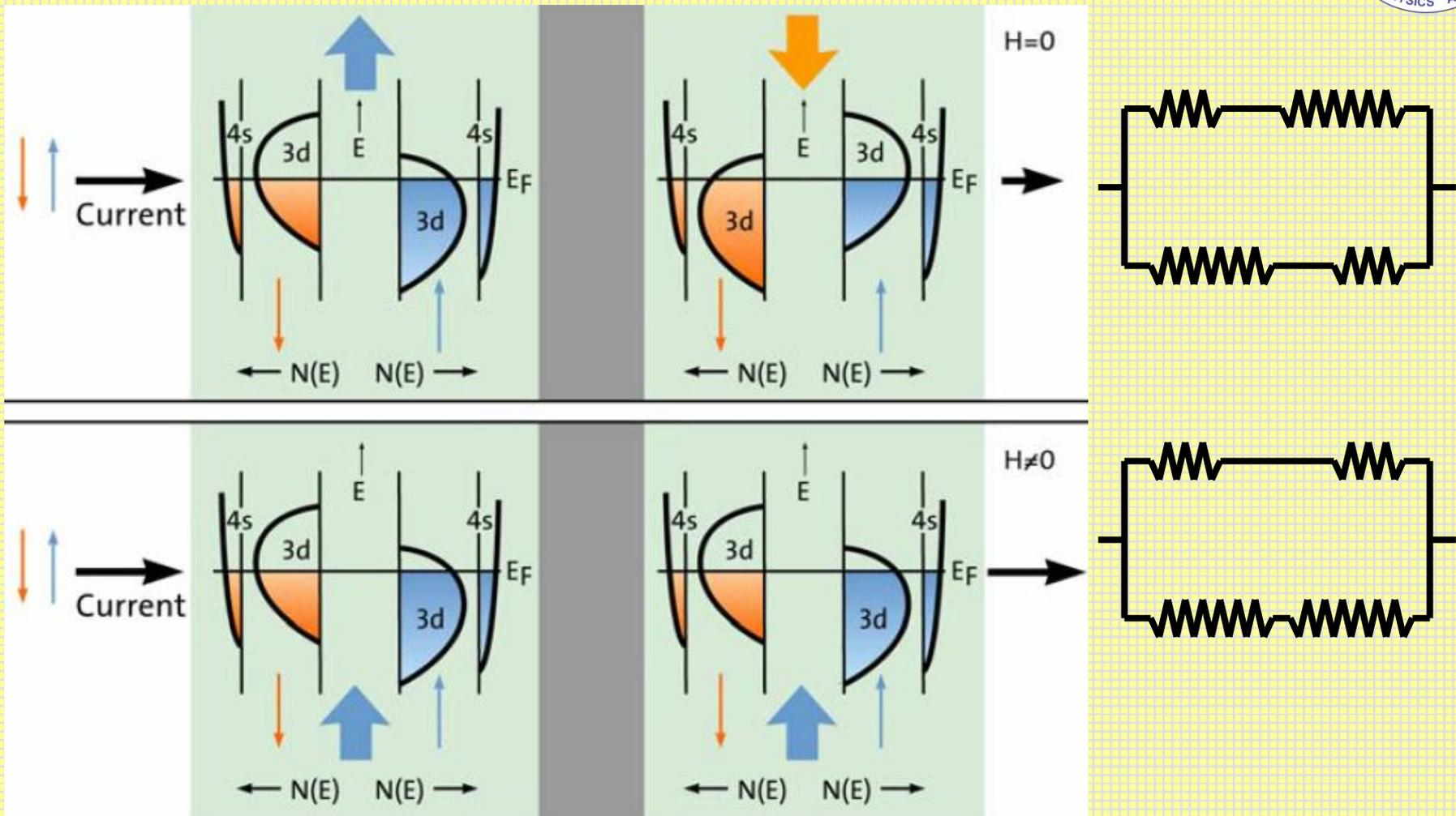
**“short circuit effect” of one spin channel results in small resistance in parallel configuration**
