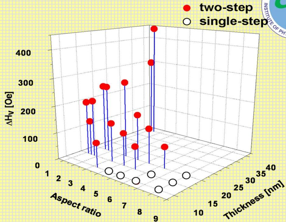
**Figure 3. Phase diagram of elliptical ring reversal behavior and the field range of the vortex state  $\Delta H_v$  as functions of the aspect ratio  $r$  and thickness  $t$  for the applied field parallel to the long axis. The solid and open circles represent two-step and single-step switching, respectively.**
