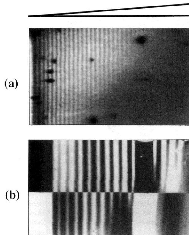
**Fig. 2.44.** The effect of roughness on the inertlayer exchange coupling is shown by a comparison of (a) the oscillations of the RHEED intensity along the bare Cr wedge with (b) the SEMPA magnetization image over the same part of the wedge
