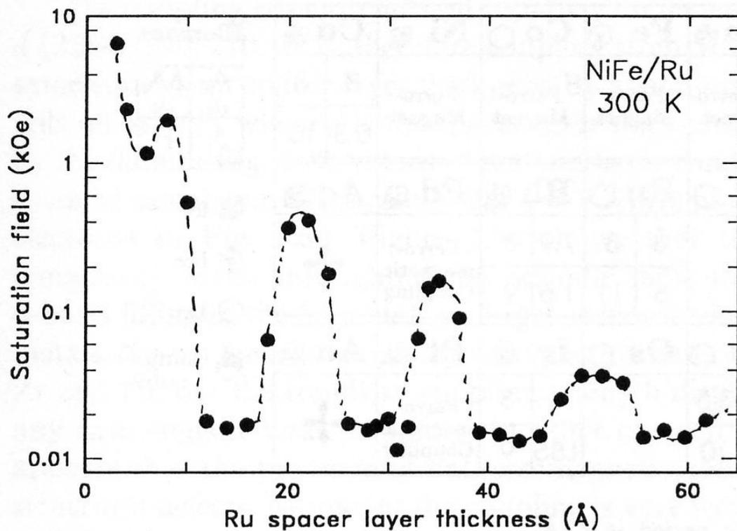
**Fig. 2.58.** Dependence of saturation field on Ru spacer layer thickness for several series of  $\text{Ni}_{81}\text{Fe}_{19}/\text{Ru}$  multilayers with structure,  $100 \text{ \AA} \text{ Ru}/[30 \text{ \AA} \text{ Ni}_{81}\text{Fe}_{19}/\text{Ru}(t_{\text{Ru}})]_{20}$ , where the topmost Ru layer thickness is adjusted to be  $\approx 25 \text{ \AA}$  for all samples
