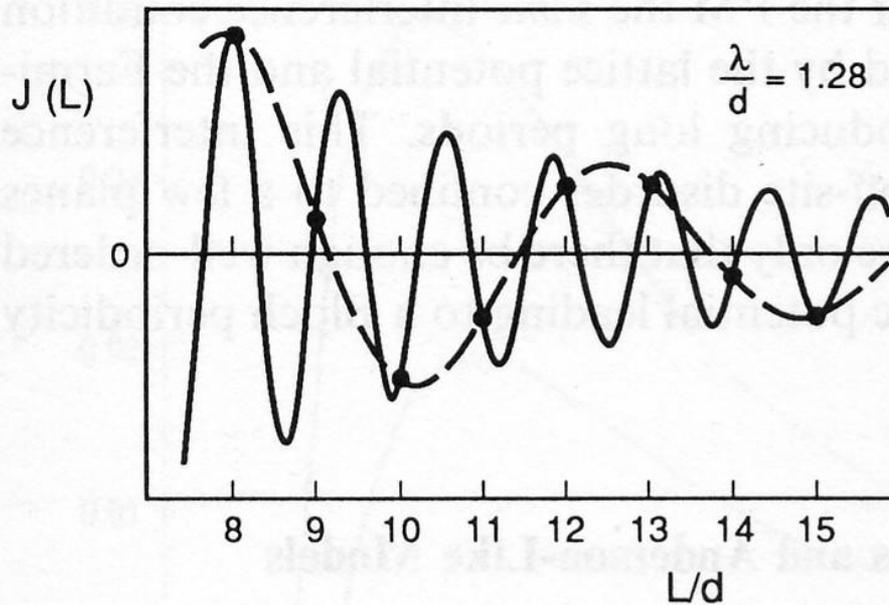
**Fig. 2.10.** RKKY-like oscillating exchange coupling with period  $\lambda$  (solid line) showing the longer period oscillation (dashed line) obtained by sampling the function only at integral values of the spacing,  $a$ , between atomic planes, i.e. “aliasing”. From [2.21]
