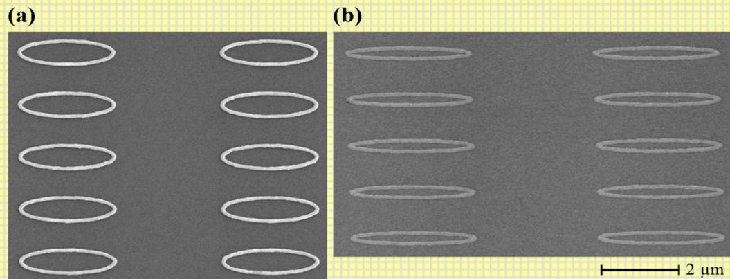
Scanning electron microscope images of selected samples (a) aspect ratio  $r=3.3$  and (b)  $r=8$  arrays of elliptical rings. The edge-to-edge distance in the long axis direction is fixed at  $3 \mu\text{m}$ .
