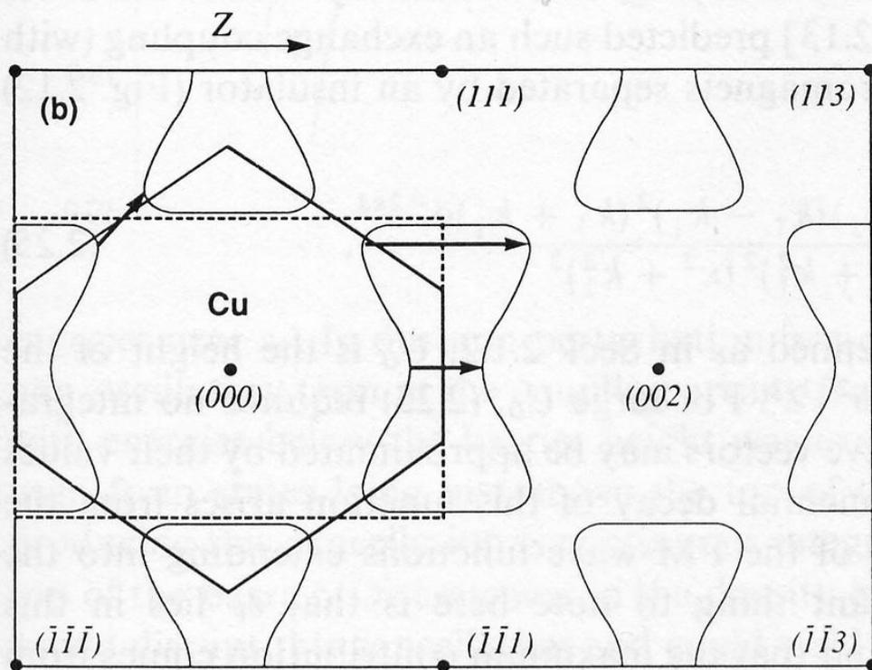
**Fig. 2.11.** Fermi surface of Cu in the (100) plane in the extended zone scheme. Arrows indicate values of  $2(k_F - G)$  for reciprocal lattice vectors  $G$  which can give rise to oscillations with periods greater than  $\pi/k_F$
