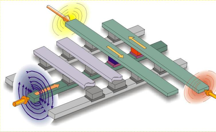
STT-RAM : «Electronic» reversal by spin transfer from an electrical current
