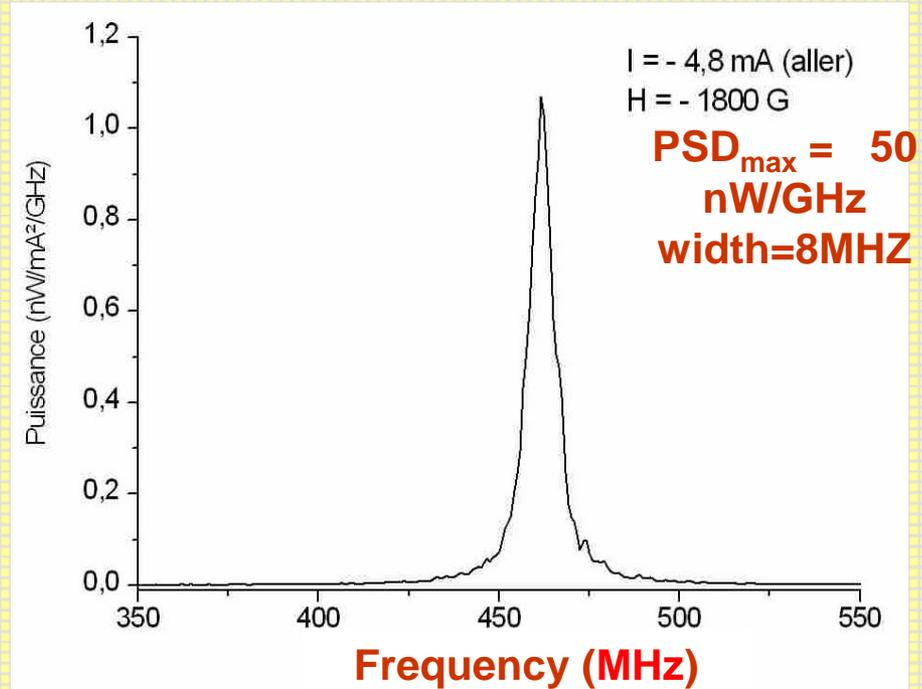
Low frequency vortex excitation in Py/Au/Co nanocontacts (CNRS/Thales, A.Ruotolo et al, 2008)
