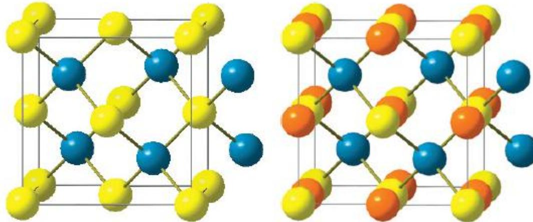
**Figure 1 | Comparison of the zinc-blende and the  $C1_b$  crystal structure.** The zinc-blende (XY) structure is shown on the left, and the  $C1_b$  (XYZ) on the right. Yellow and blue spheres correspond to the main-group (Z) and transition (Y) elements, respectively. The orange spheres in  $C1_b$  stand for the additional stuffing (X) element.
