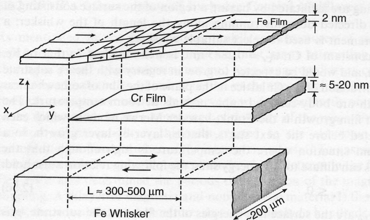
**Fig. 2.41.** A schematic expanded view of the sample structure showing the Fe(001) single-crystal whisker substrate, the evaporated Cr wedge, and the Fe overlayer. The arrows in the Fe show the magnetization direction in each domain. The  $z$ -scale is expanded approximately 5000 times. (From [2.206])
