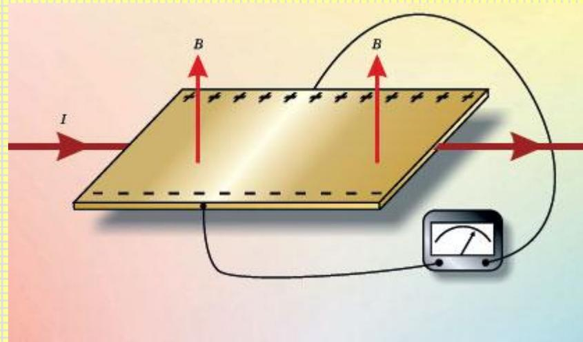
Edwin Hall's 1878 experiment was the first demonstration of the Hall effect. A magnetic field  $B$  normal to a gold leaf exerts a Lorentz force on a current  $I$  flowing longitudinally along the leaf. That force separates charges and builds up a transverse "Hall voltage" between the conductor's lateral edges. Hall detected this transverse voltage with a voltmeter that spanned the conductor's two edges.
