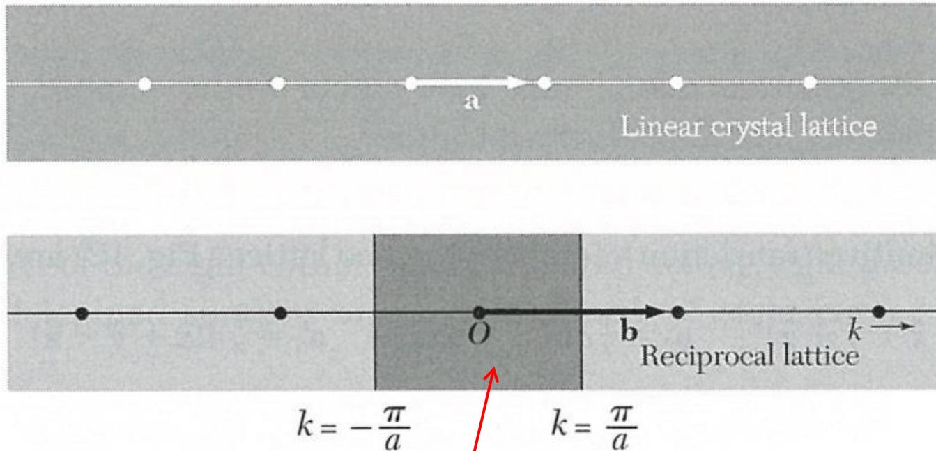
**Figure 11** Crystal and reciprocal lattices in one dimension. The basis vector in the reciprocal lattice is **b**, of length equal to  $2\pi/a$ . The shortest reciprocal lattice vectors from the origin are **b** and **-b**. The perpendicular bisectors of these vectors form the boundaries of the first Brillouin zone. The boundaries are at  $k = \pm\pi/a$ .
