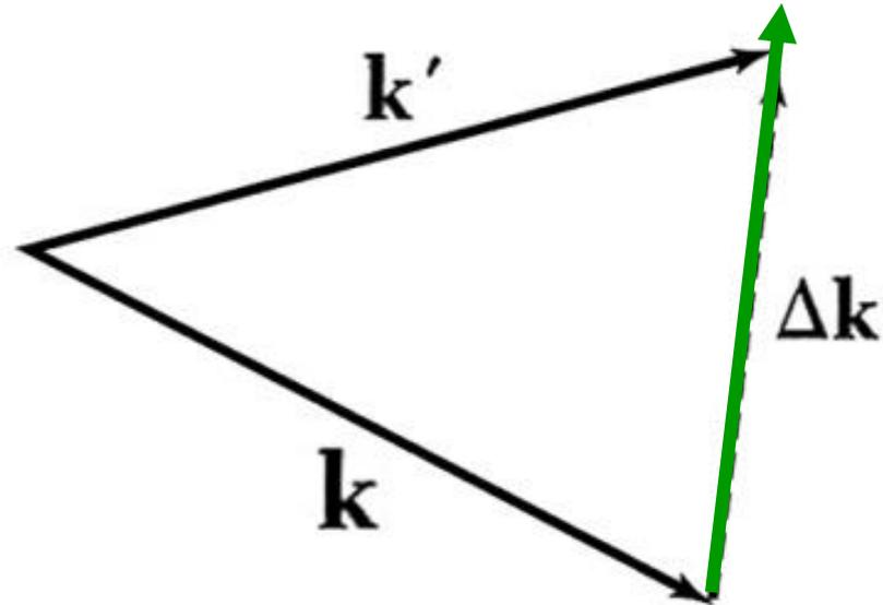
**Figure 7** Definition of the scattering vector  $\Delta\mathbf{k}$  such that  $\mathbf{k} + \Delta\mathbf{k} = \mathbf{k}'$ . In elastic scattering the magnitudes satisfy  $k' = k$ . Further, in Bragg scattering from a periodic lattice, any allowed  $\Delta\mathbf{k}$  must equal some reciprocal lattice vector  $\mathbf{G}$ .
