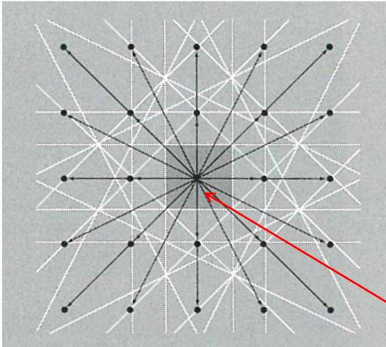
**Figure 9b** Square reciprocal lattice with reciprocal lattice vectors shown as fine black lines. The lines shown in white are perpendicular bisectors of the reciprocal lattice vectors. The central square is the smallest volume about the origin which is bounded entirely by white lines. The square is the Wigner-Seitz primitive cell of the reciprocal lattice. It is called the first Brillouin zone.
