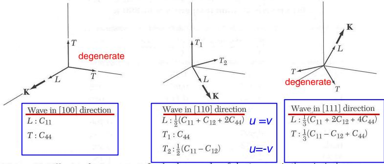
**Figure 20** Effective elastic constants for the three modes of elastic waves in the principal propagation directions in cubic crystals. The two transverse modes are degenerate for propagation in the [100] and [111] directions.
