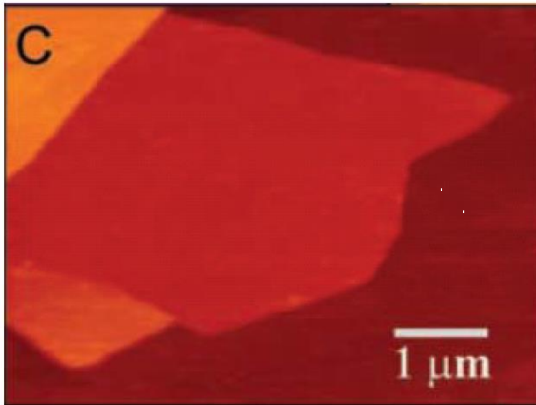
mechanically exfoliated graphene sheets
