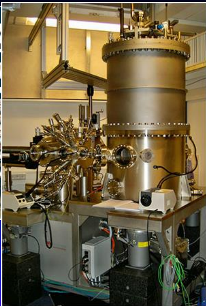
➤ Home built 4K-STM with 3D Magnets
