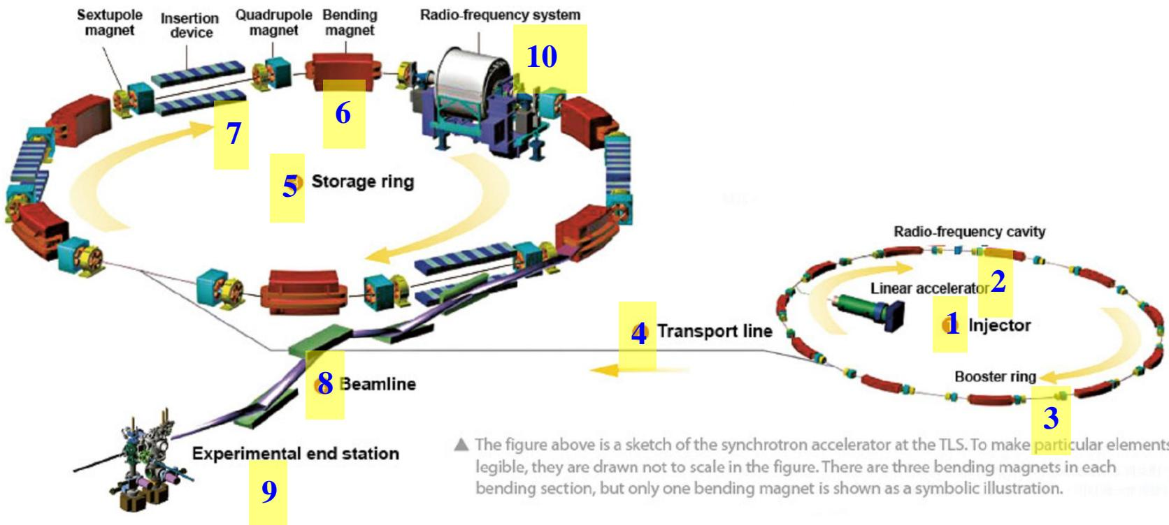
▲ The figure above is a sketch of the synchrotron accelerator at the TLS. To make particular elements legible, they are drawn not to scale in the figure. There are three bending magnets in each bending section, but only one bending magnet is shown as a symbolic illustration.
