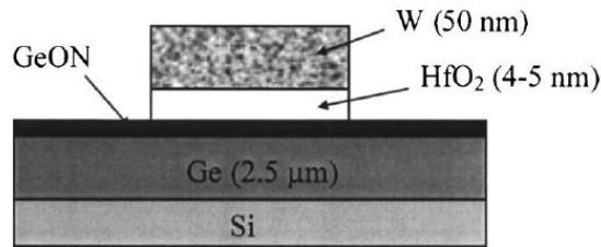
FIG. 1. Diagram of the W/HfO<sub>2</sub>/GeON/Ge stack.
