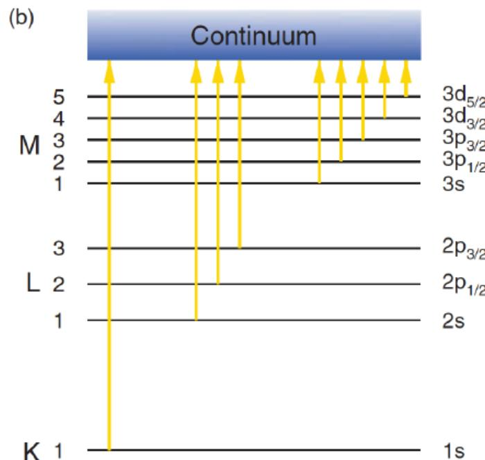
**Figure 2.16** (a) The x-ray absorption coefficient  $\mu$  for beryllium (red curve), silicon (yellow) and lead (blue) as a function of the photon energy. (b) Sharp increases in the absorption occur when the photon energy is just sufficient to eject the electron from the electronic orbital to the continuum. The x-ray absorption (left) and atomic orbital labellings (right) are shown.
