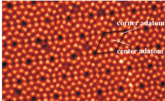
Si(111)-(7x7),  $V_s = 1.6$  V,  $I = 1$  nA, Scanning Size = 12.5 nm x 20.5 nm
