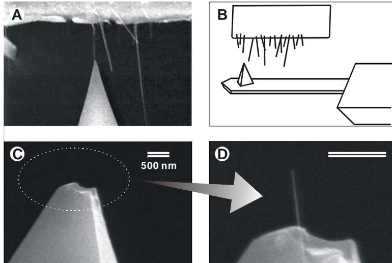
Carbon nanotube: The ultimate probe for imaging long-range forces?
