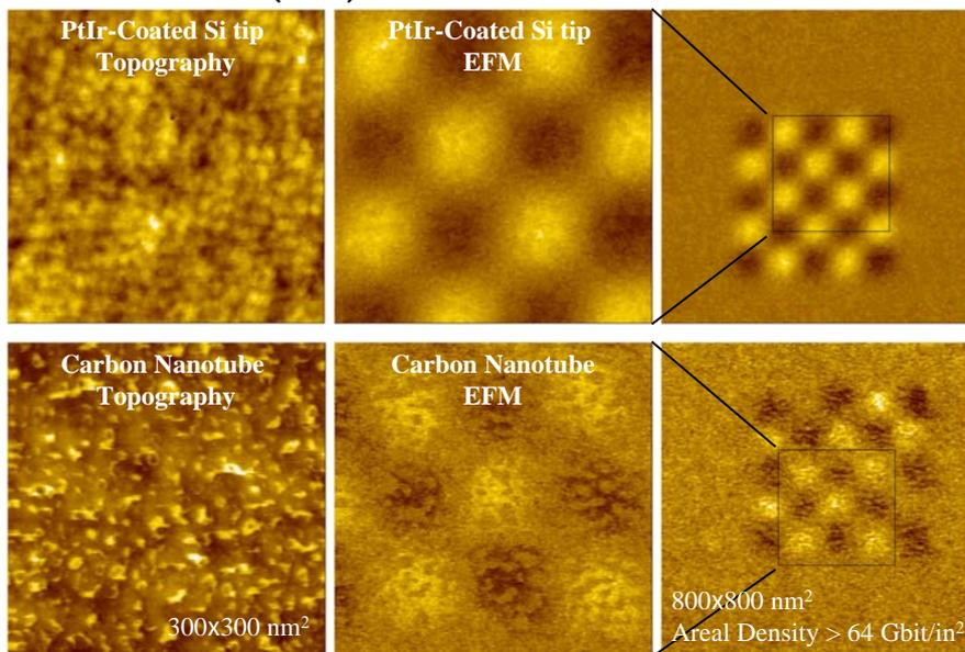
Charging conditions:  $\pm 10$  V voltage pulses (1-ms pulse-width for PtIr-coated Si tip, 1-s pulse-width for CNT tip)
