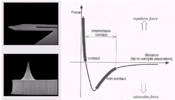
Fig. 13. Piezolever™, ThermoMicroscopes AutoProbe, contact mode (left), interatomic forces (right).
