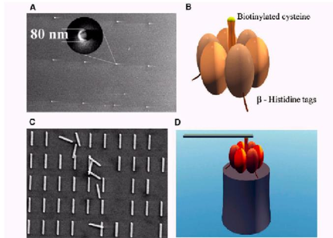
**Fig. 1.** Schematic diagram of the F<sub>1</sub>-ATPase biomolecular motor-powered nanomechanical device. The device consisted of (A) a Ni post (height 200 nm, diameter 80 nm), (B) the F<sub>1</sub>-ATPase biomolecular motor, and (C) a nanopropeller (length 750 to 1400 nm, diameter 150 nm). The device (D) was assembled using sequential additions of individual components and differential attachment chemistries.
