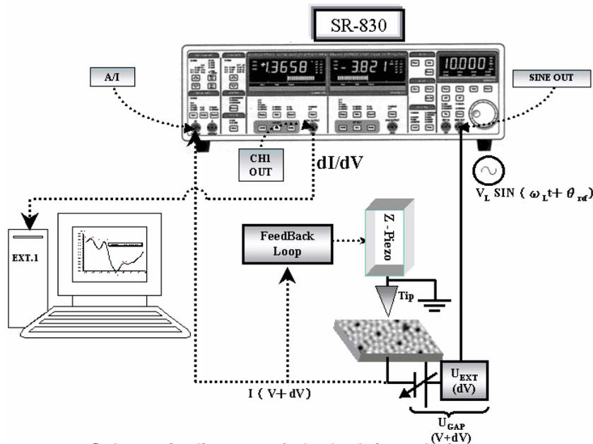
**Schematic diagram of the lock-in technique**
