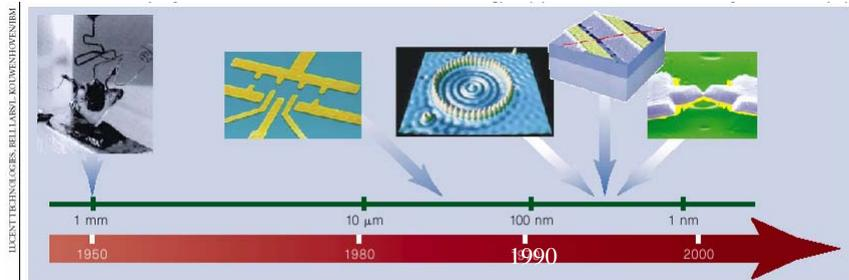
Figure 1 The shrinkage of electronic components. The length scale reached by technology has dropped steadily from the millimetre scale of the early 1950s to the present-day atomic scale. The representative devices, from left to right, are: the first transistor, a quantum-dot turnstile, a copper 'quantum corral', a carbon-nanotube transistor, and the latest — a one-atom point contact.
