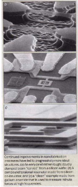
Continued improvements in nanofabrication processes have led to progressively more ideal structures. (a) An early (and rather rough) doubly clamped beam "carved" from a silicon wafer. (b) A compound torsional resonator made from silicon-on-insulator, and (c) a "clean" example made from gallium arsenide that is used to measure minute forces at high frequencies.
