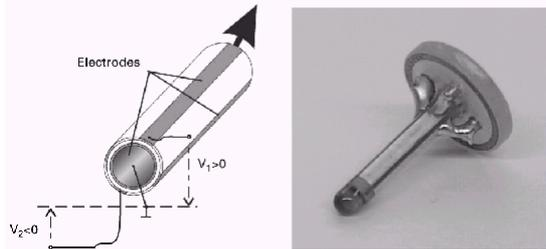
Fig. 3. Piezoelement with segmented electrodes (left), piezoleg with ruby ball (right).
