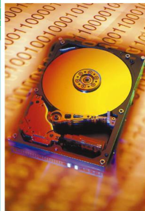
Well read: spintronics has dramatically increased data storage densities in hard drives.
