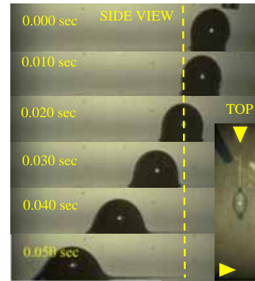
2 \mu\text{L} water droplet, \psi = 4^\circ , and L=12\text{ mm}
