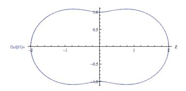
The total power is given by integration over angles. The result is  $P = \frac{2e^2R^2\omega_0^4}{3c^3}$ .
