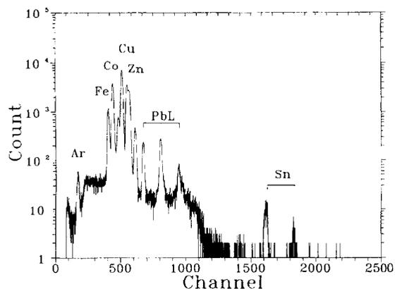
Fig. 1. PIXE spectrum of the Wan-lih coin (sample 39) obtained by 3 MeV proton beam bombardment on the surface of the coin at one irradiation. The observed Co peak is induced by the fluorescence in the absorber inserted between the target and the detector.
