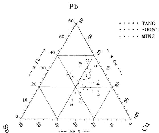
Fig. 2. Ternary diagram of Cu, Pb and Sn concentrations for the 35 bronze coins (samples 1 to 35) of various periods. Data points are plotted as the percent by weight of each element with the normalization  $Cu + Pb + Sn = 1$ .
