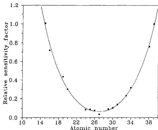
Fig. 2. A plot of relative sensitivity factor  $\eta$  as the function of atomic number  $Z$ , obtained for the detection system used in the present PIXE measurements.
