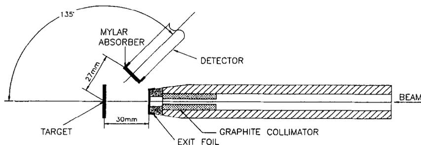
Fig. 1. Experimental setup for the external-beam PIXE measurement.
