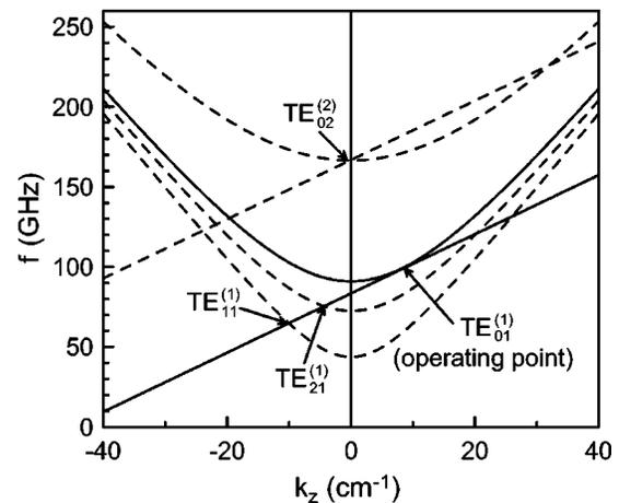
FIG. 1. Frequency vs  $k_z$  diagrams of the waveguide modes and the beam-wave synchronism lines for a  $TE_{01}$ -mode, 94-GHz gyro-TWT operating at the fundamental cyclotron harmonic. Parameters used are (see also Table I): waveguide radius=0.201 cm, beam voltage=100 kV, velocity ratio ( $v_{\perp}/v_z$ )=1.0, and  $B_0=35.6$  kG. The applied magnetic field  $B_0$  is set at 0.995 of the grazing value ( $B_{g01}=35.8$  kG) for the operating mode.
