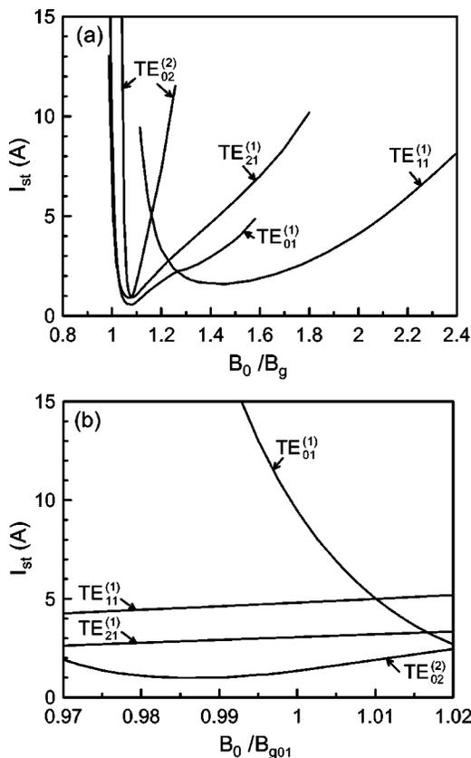
FIG. 7. (a) Start-oscillation currents versus  $B_0/B_g$ , where  $B_g$  is the grazing magnetic of the respective mode. In this figure, different modes are displayed on different absolute magnetic field scales. (b) Start-oscillation currents plotted on the same absolute magnetic field scale over a narrow range around the grazing magnetic field of the operating mode  $B_{g01}$ .
