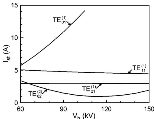
FIG. 8. Start-oscillation currents versus the beam voltage  $V_b$ .
