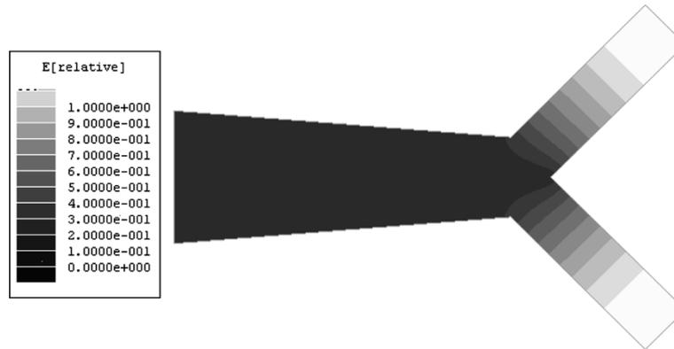
Fig. 5. Normalized electric field patterns of the first two resonant modes under study obtained using HFSS. (a) Fundamental mode and (b) first high-order mode. The electric fields of the two wings in the fundamental mode are in phase, while in the first high-order mode, they are out of phase, and the central stem is not excited.
