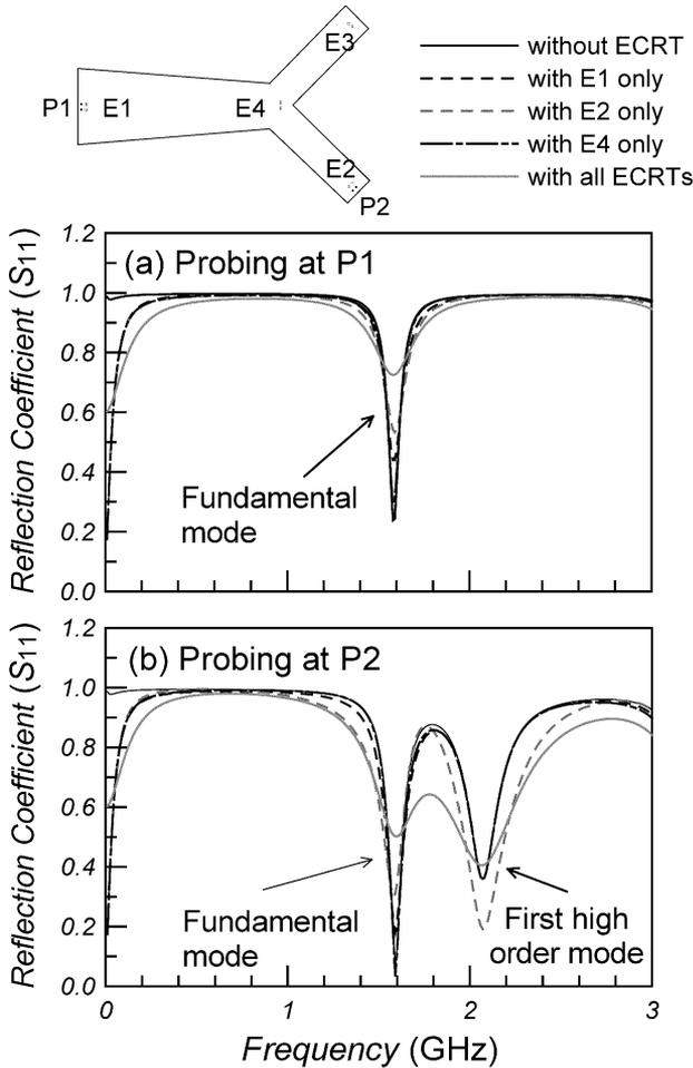
Fig. 6. Speed2000 simulation results concerning the reflection coefficient (a) when probes at P1 with P2 disabled and (b) when probes at P2 with P1 disabled, given various ECRT configurations. In both modes, as expected, with no ECRT, the quality factors are highest, whereas with all ECRTs present, the quality factors are lowest.
