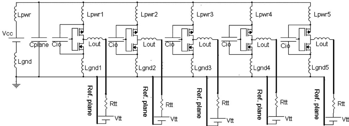
Fig. 3. Equivalent SPICE model of five CMOS buffers. A VCR model is employed to represent the CMOS to study the frequency response. This illustration is used to clarify how the I/O buffer is modeled.
