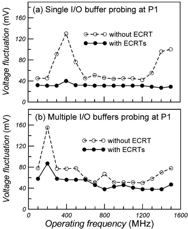
Fig. 9. Maximum voltage fluctuation detected at the end of the central stem, P1, without ECRT (dashed lines with open circles) and with ECRT (solid lines with closed dots) for (a) single and (b) multiple I/O buffers.
