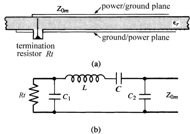
Fig. 4. (a) Structure and (b) the equivalent circuit of the ECRT under study. The central post is not in physical contact with the other hetero plane. Therefore, it does not affect the dc voltage, but damps RF noise as can be seen in the equivalent circuit. In practice, the whole ECRT circuit is made ready using the existing via plus a termination resistor.
