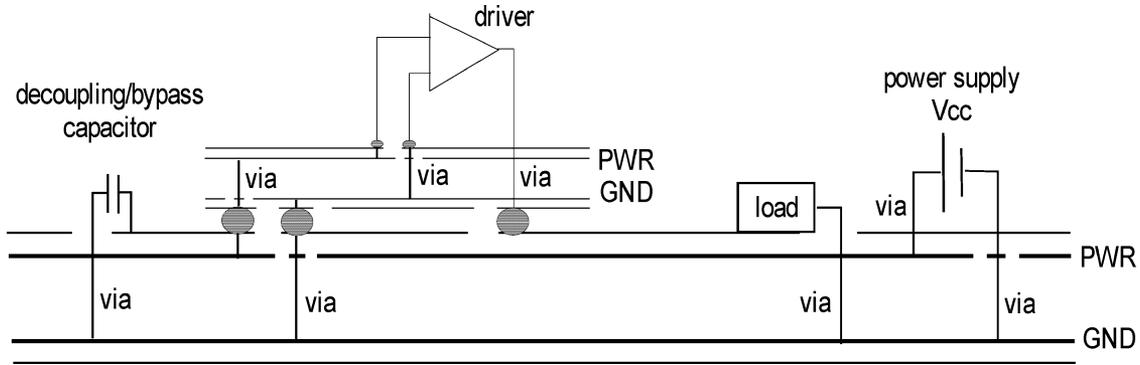
Fig. 1. Schematic diagram of the power distribution network. The I/O buffer draws its energy from a far-end power supply. The decoupling capacitor in the vicinity of the driver shortens the effective power delivery loop and compensates the voltage drop during transition.
