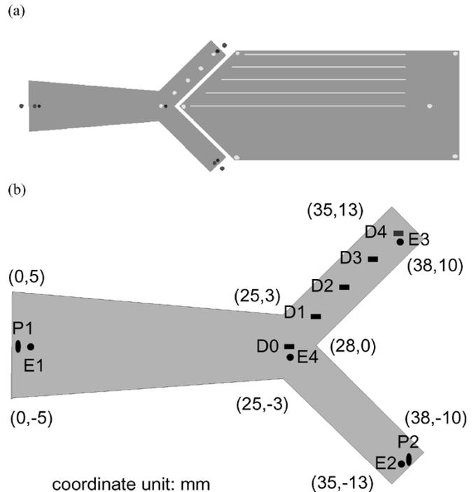
Fig. 2. (a) Top view of the second layer (L2), showing the power plane (Y-shaped) and the ground plane (pentagon). The traces and connecting pads on the Signal 1 layer are also projected. The third layer (L3) is a ground plane. (b) Position of the I/O buffers (denoted by D0 to D4), the detecting points (P1 to P2), and the external coupled resistive termination (ECRT) circuits (E1 to E4). The coordinates are in millimeters.
