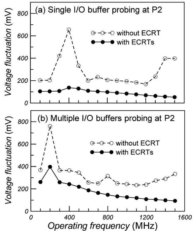
Fig. 8. Maximum voltage fluctuation detected at the end of one wing, P2, without ECRT (dashed lines with open circles) and with ECRT (solid lines with closed dots) for (a) single and (b) multiple I/O buffers.
