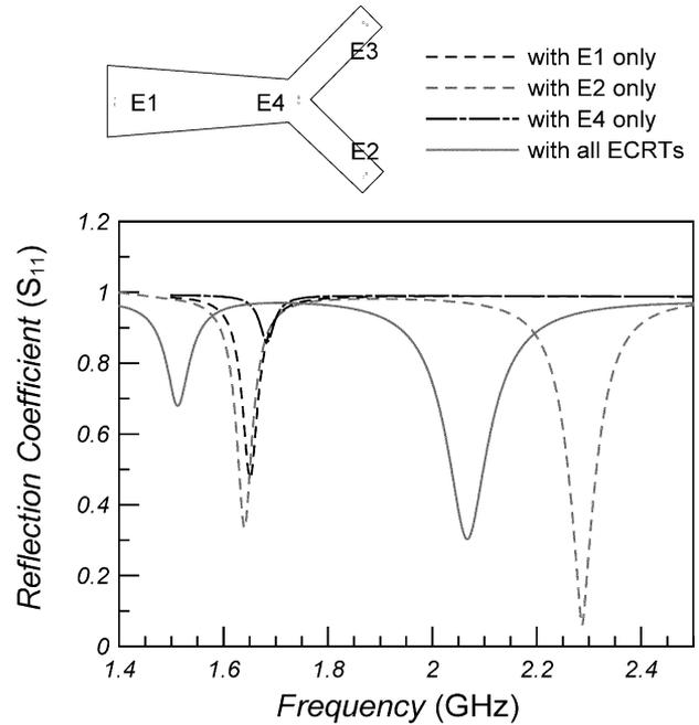
Fig. 7. HFSS simulation results; the reflection coefficients are obtained by treating each ECRT circuit as a coaxial port. Placing the ECRT close to the field bulk affects the resonant frequency and lowers the quality factor. The characteristic impedance of the coaxial port of the ECRT is not optimized.
