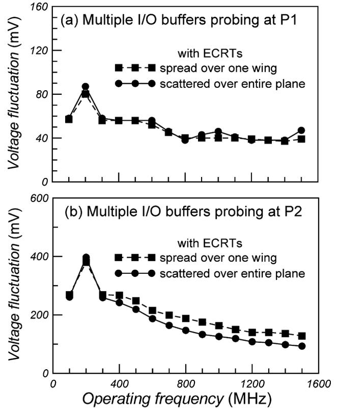
Fig. 10. Maximum voltage fluctuation for two placement configurations of the ECRT. The switching noise when the ECRTs are uniformly spread over one wing is represented by dashed lines with squares, while that when the ECRTs are scattered over the entire plane, as in Fig. 2(b), are represented by solid lines with dots. The results detected (a) at P1 and (b) at P2 are displayed.
