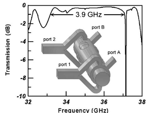
FIG. 9. Calculated back-to-back transmission with extra ports (ports A and B). These extra ports are used to absorb the degenerate  $TE_{21}$  wave. The calculated 1-dB bandwidth is 3.9 GHz, which is the same as the single converter's prediction.
