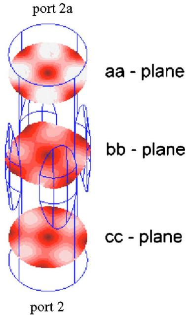
FIG. 4. (Color online) The cross section of the electric field distribution at three different planes: aa plane (linear polarization, before), bb plane (elliptical polarization, middle), and cc plane (circular polarization, after).
