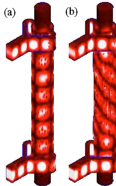
FIG. 5. (Color online) The electric field strengths simulated with HFSS for (a) two identical linearly polarized converters joining back to back, and (b) two identical circularly polarized converters joining back to back.
