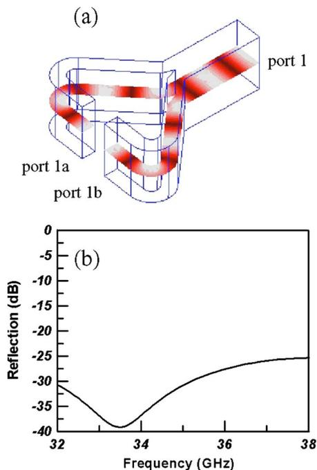
FIG. 2. (Color online) The HFSS simulation results. (a) The distribution of the electric field strength of the power-dividing section, viewed at the middle cross section of the rectangular waveguide. (b) The frequency response of the reflection at port 1, where ports 1a and 1b are assumed to be matched to elude the multiple reflections effect.
