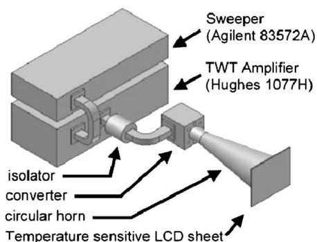
FIG. 10. The schematic diagram of the experimental setup of directly measuring the field distribution pattern. The rf power, generated by a TWT and controlled by a sweeper/synchronizer, is injected into the mode converter. A sheet of temperature-sensitive LCD is placed in front of the circular horn, where the color spectrum is proportional to the electric field strength.
