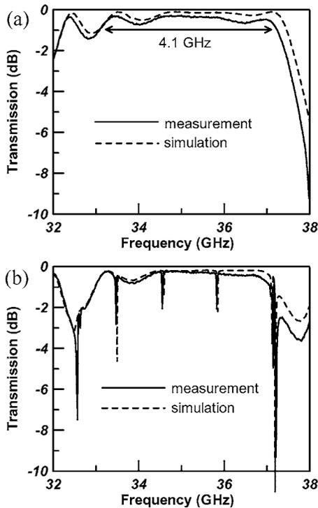
FIG. 7. The calculated and measured transmission loss for two identical converters joining back to back: (a) linear polarization and (b) circular polarization.
