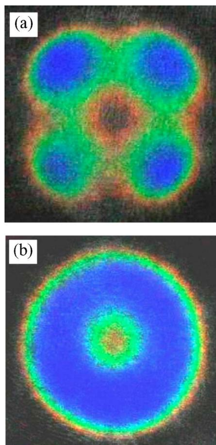
FIG. 11. (Color online) The measured time-averaged field distribution on the LCD sheet for (a) a linearly polarized TE<sub>21</sub> wave, and (b) a circularly polarized TE<sub>21</sub> wave.
