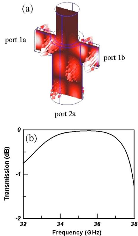
FIG. 3. (Color online) (a) The cross section of the electric field distribution with HFSS. (b) The frequency response of the transmission from two rectangular  $TE_{10}$  modes to the circular  $TE_{21}$  mode.
