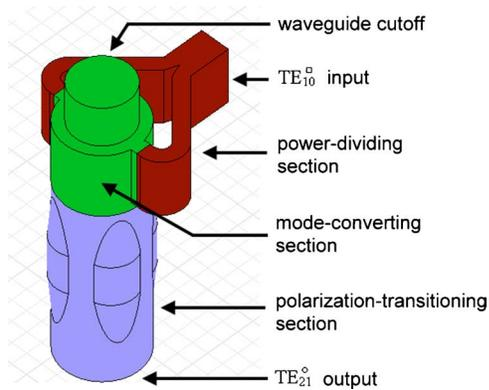
FIG. 1. (Color online) The schematic diagram of the  $TE_{21}$  mode and polarization converter under study. The mode-converting processes consist of three stages: the power-dividing section, the mode-converting section, and the polarization-transitioning section.
