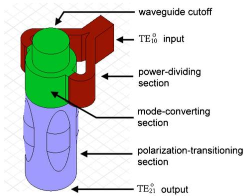
FIG. 1. (Color online) The schematic diagram of the  $TE_{21}$  mode and polarization converter under study. The mode-converting processes consist of three stages: the power-dividing section, the mode-converting section, and the polarization-transitioning section.
