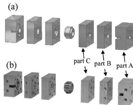
FIG. 6. (a) The design drawing of the parts of the two identical converters. A circular polarization converter operating at the Ka band with a center frequency of 35.0 GHz is to be built. (b) The finished parts, which are made of copper and are machined with a CNC lathe with a tolerance of 0.01 mm. Pins are used to enhance the alignment.
