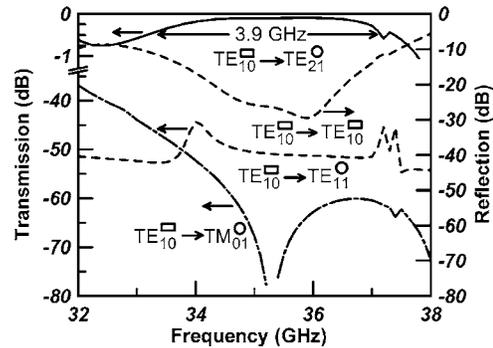
FIG. 8. Calculated transmission loss and reflection loss vs frequency for a single circular polarization mode converter. The transmission loss from a rectangular waveguide mode to three cylindrical waveguide modes,  $TE_{21}$ ,  $TE_{11}$ , and  $TM_{01}$ , are displayed. The left y axis is broken to display the excellent  $TE_{21}$  mode conversion. A 0.5-dB transmission bandwidth is 3.9 GHz.
